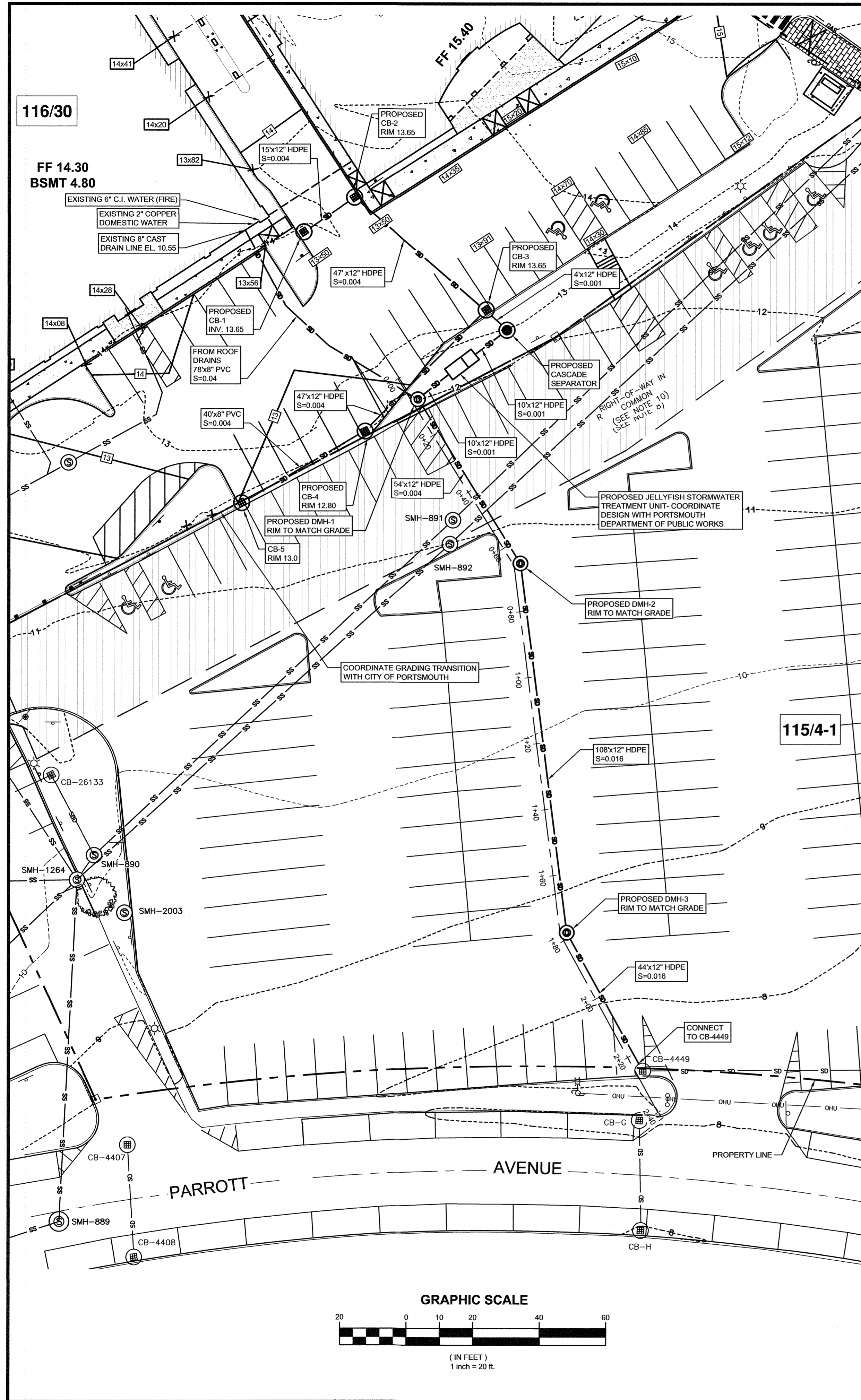
PROFILE VIEW OF PROPOSED SITE DRAINAGE TO PARROTT AVE. - STA 0+00 TO 2+40 SCALE: H: 1"=20' / V: 1"=5'
