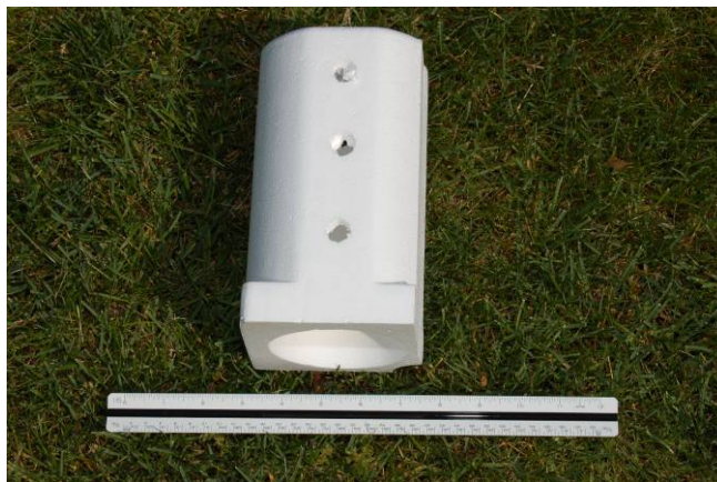
Figure 2 - Styrofoam cylinders used for temperature measurements
