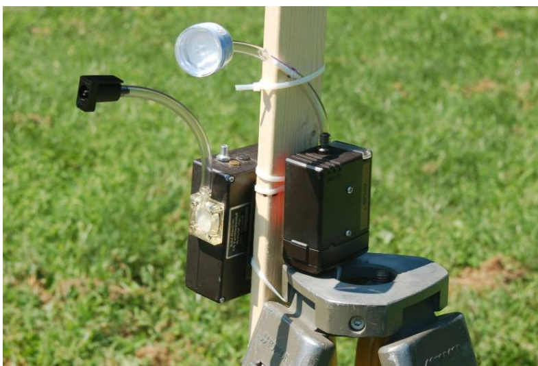
Figure 5 - Sampling Pumps. ThermoSorb N module on left; XAD-2 and filter on right
