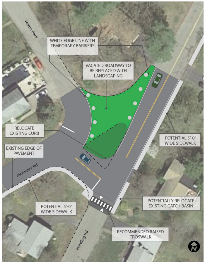
Conceptual design concept of the McKinley Road/ Harding Road intersection illustrating revised roadway geometry, new green space, and the new sidewalk with raised crosswalk
