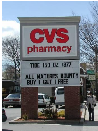
Total width of supports is greater than 1/3 of the width of the sign – Included in sign area
