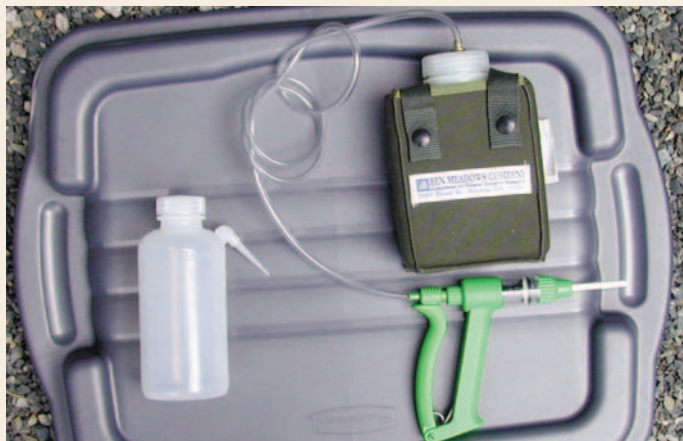
Hollow stem injection tools.
