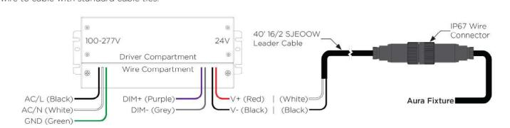
Suitable for indoor or outdoor use. Horizontal or vertical mounting. End and side knockout locations of 7/8" (1/2" trade size"). When installing multiple power supplies, separate the enclosures by at least 3" of space from edge to edge to prevent a rise of ambient temperature between the power supplies.
