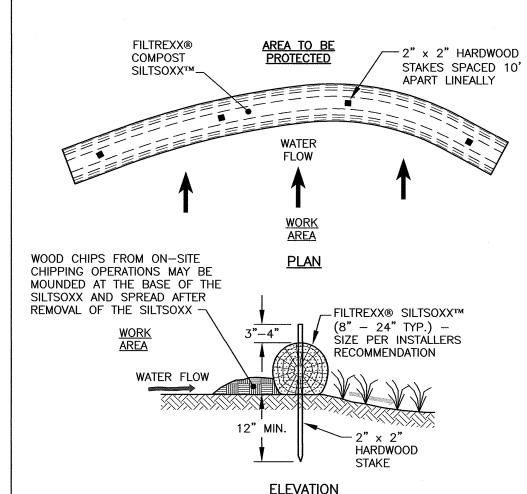
ALL MATERIAL TO MEET FILTREXX SPECIFICATIONS. FILLTREXX SYSTEM SHALL BE INSTALLED BY A CERTIFIED
