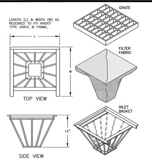
1) INLET BASKETS SHALL BE INSTALLED IMMEDIATELY AFTER CATCH BASIN CONSTRUCTION IS COMPLETE AND SHALL REMAIN IN PLACE AND BE MAINTAINED UNTIL PAVEMENT BINDER COURSE IS COMPLETE.
