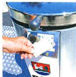
Electronic Access Control
