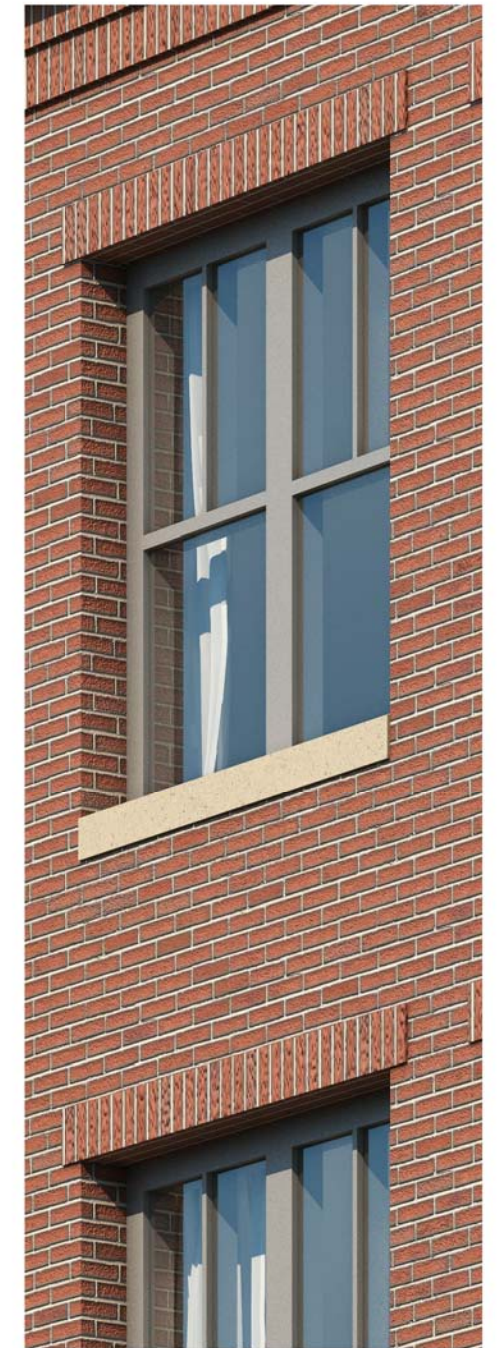
3 HEAD DETAIL - BRICK LINTEL 3/4" = 1'-0"
