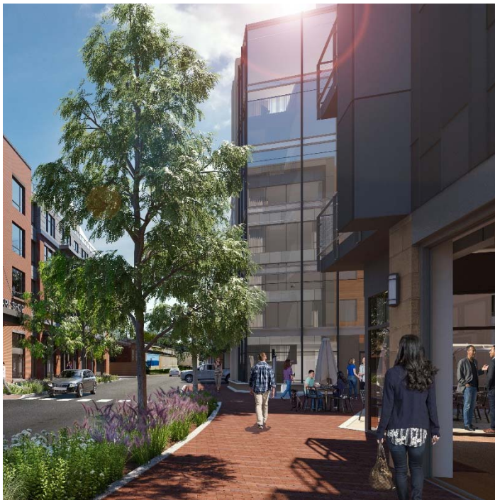
View of proposed streetscape along Foundry Way standing on the sidewalk looking towards the garage shows the planted edge to take up grade changes provide stormwater treatment and soften the pavement and building.
