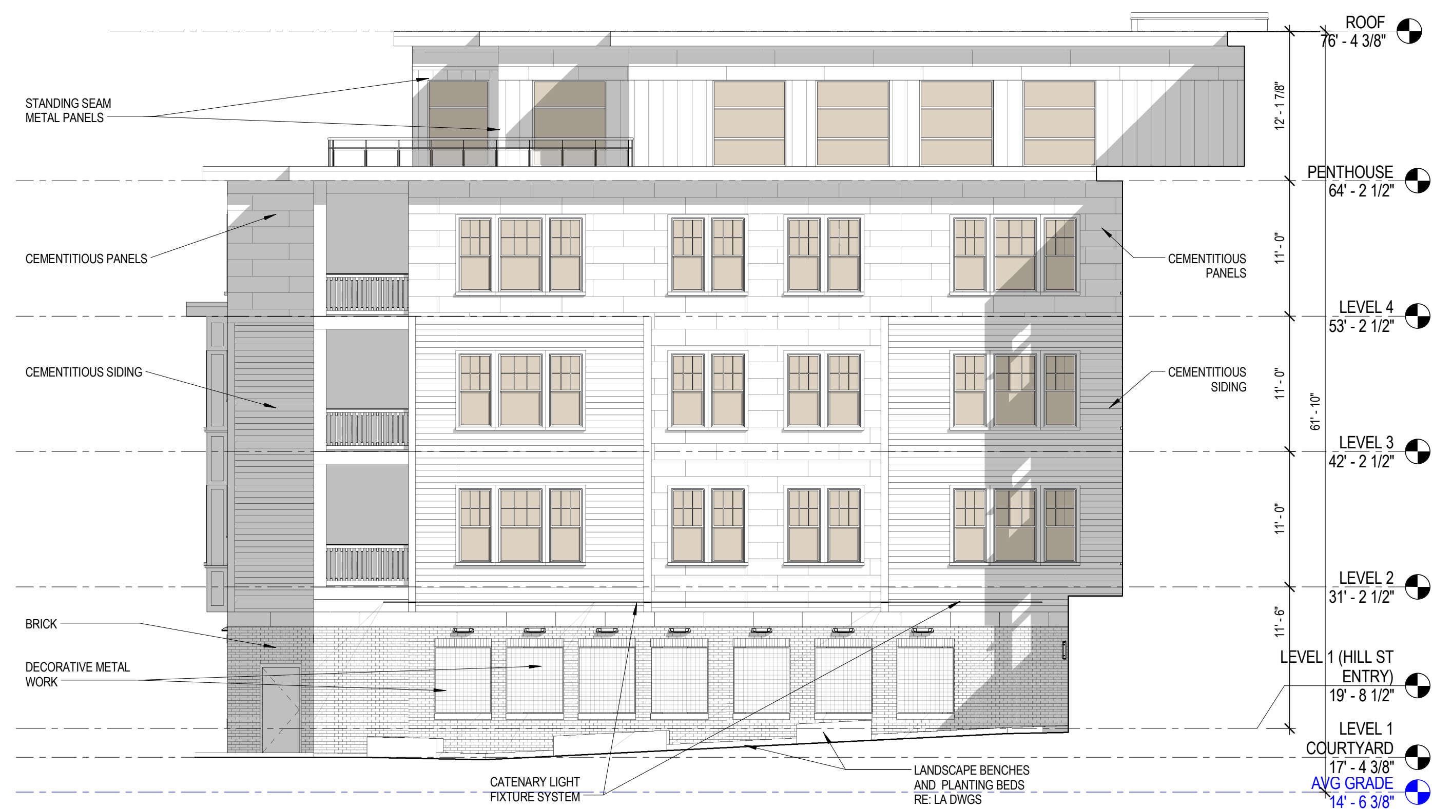
3 COURTYARD EAST ELEVATION 1/8" = 1'-0"
