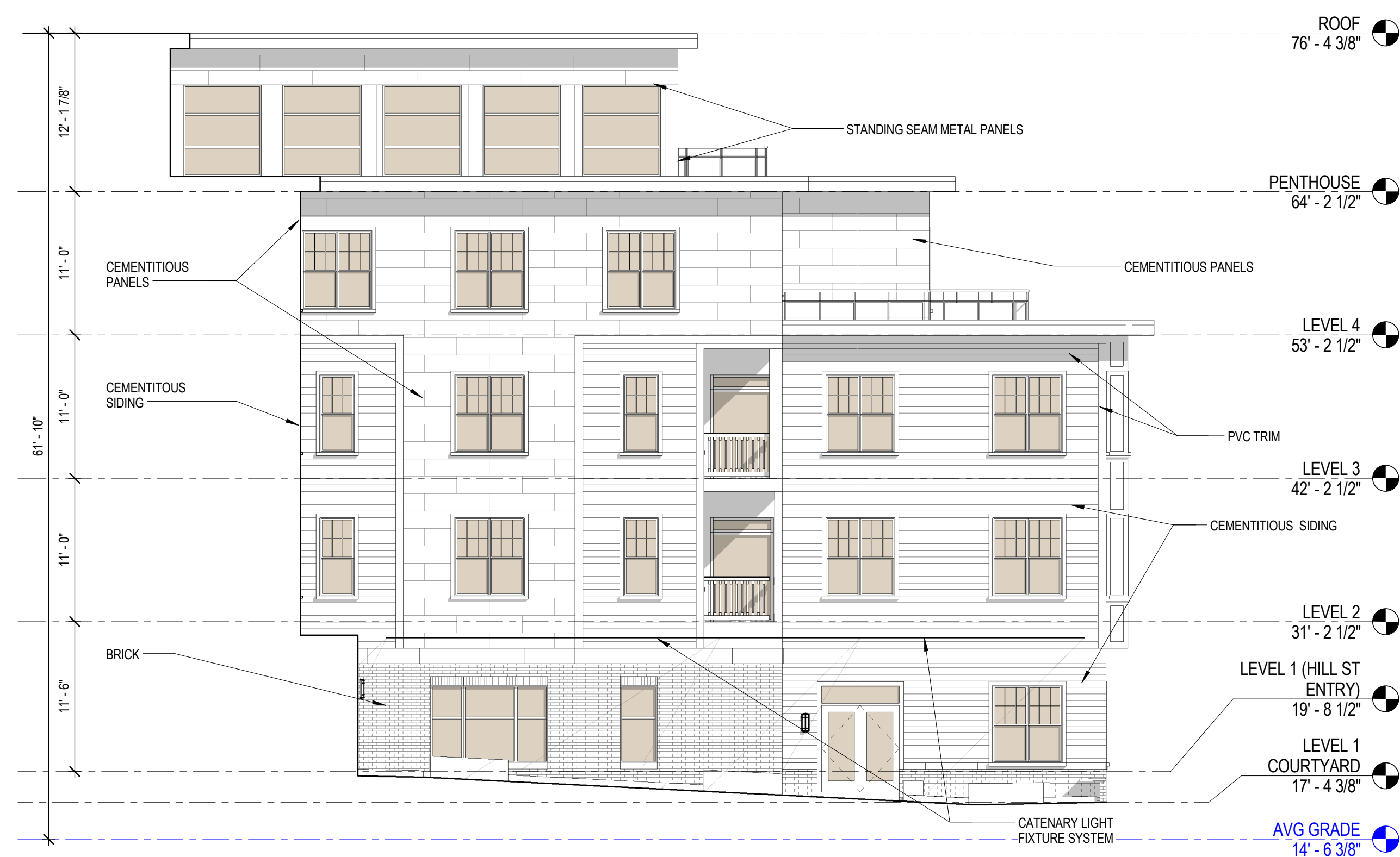
2 COURTYARD WEST ELEVATION 1/8" = 1'-0"
