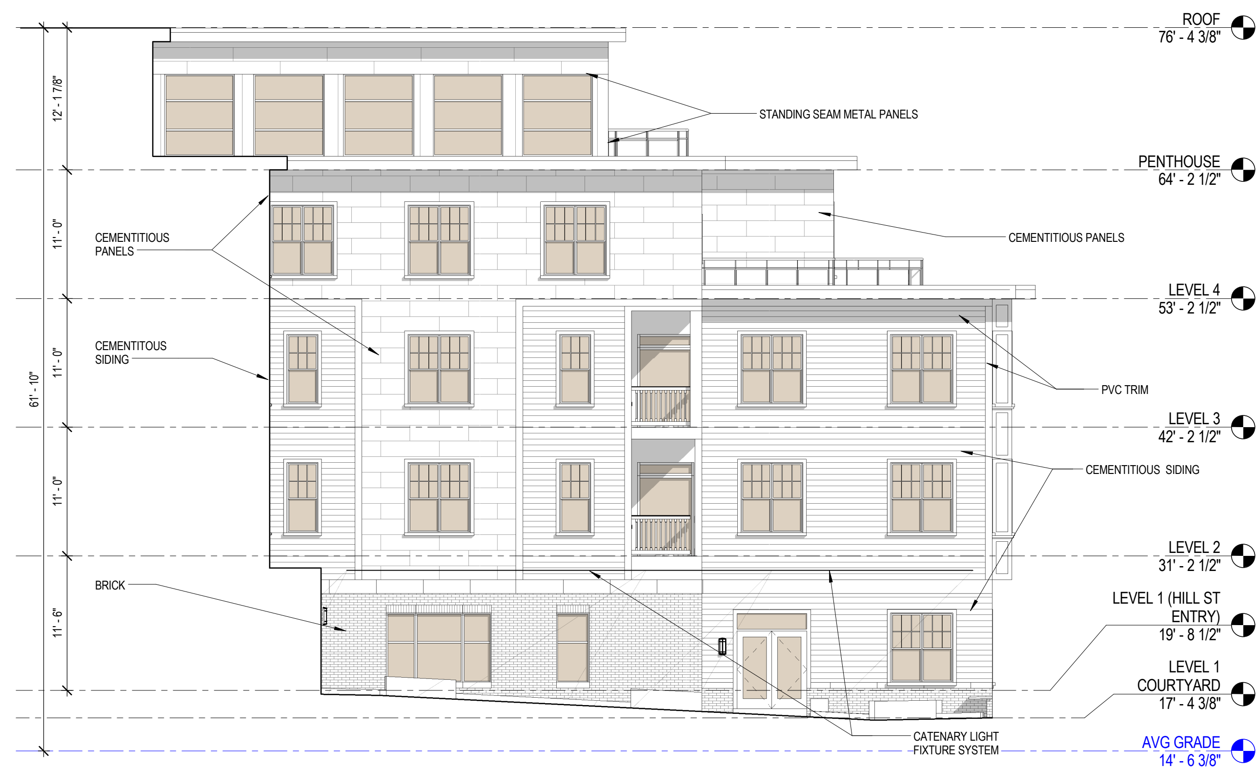
2 COURTYARD WEST ELEVATION 1/8" = 1'-0"
