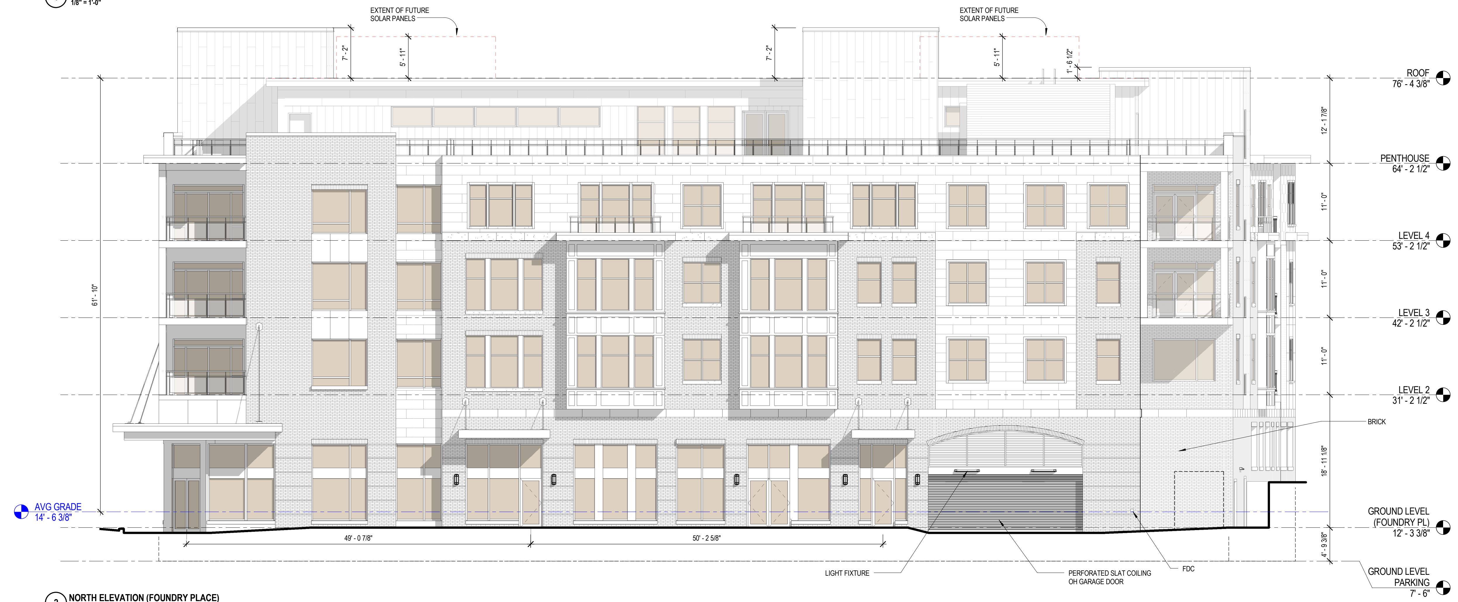
2 NORTH ELEVATION (FOUNDRY PLACE) 1/8" = 1'-0"
