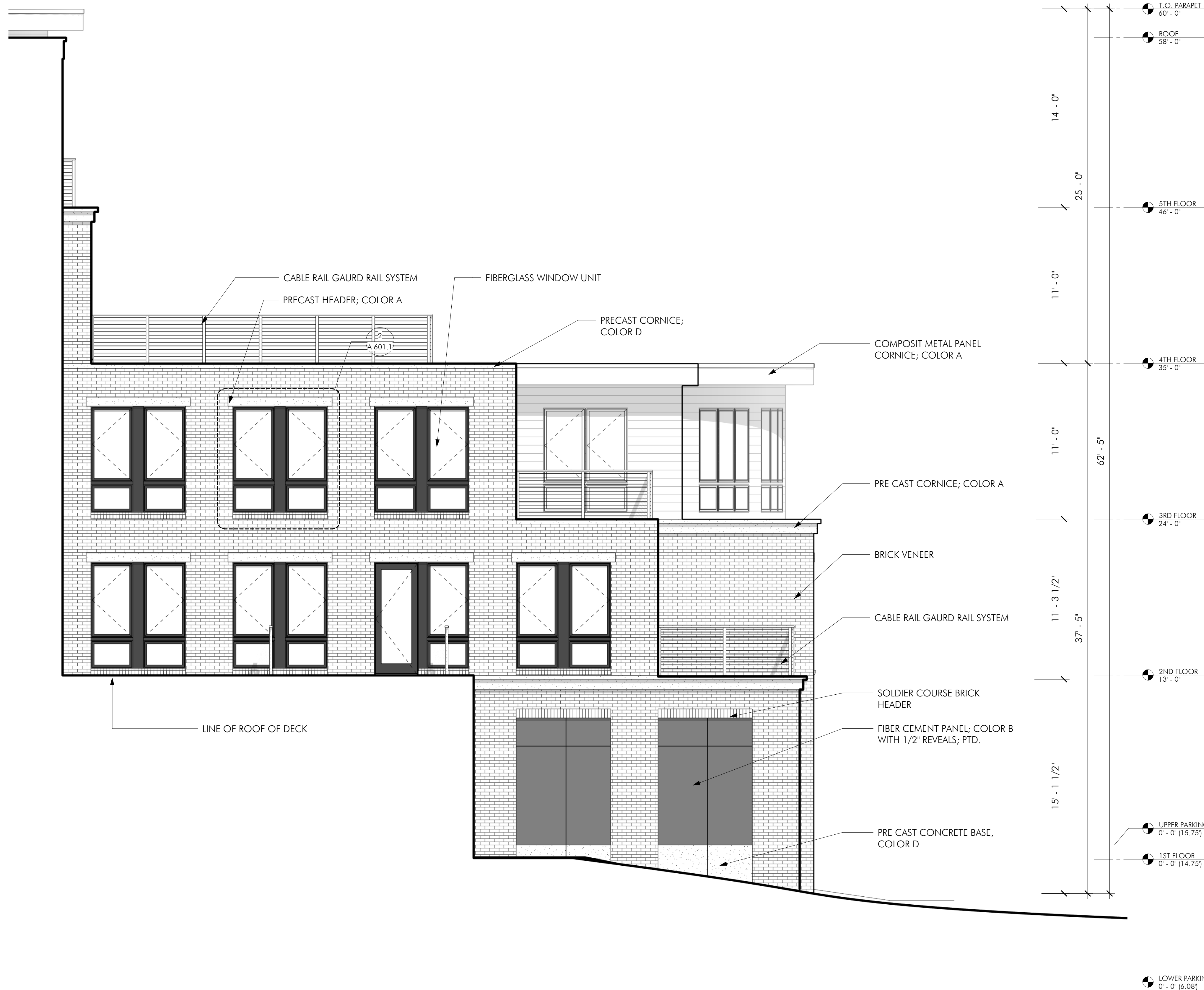
1 EAST ELEVATION (WING) 1/4" = 1'-0"
