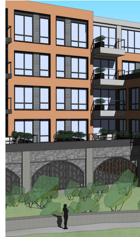
PROJECTING BALCONIES ABOVE. SOLID TEXTURED BASE ELEMENTS WITH HORIZONTAL AND VERTICAL BANDING.
