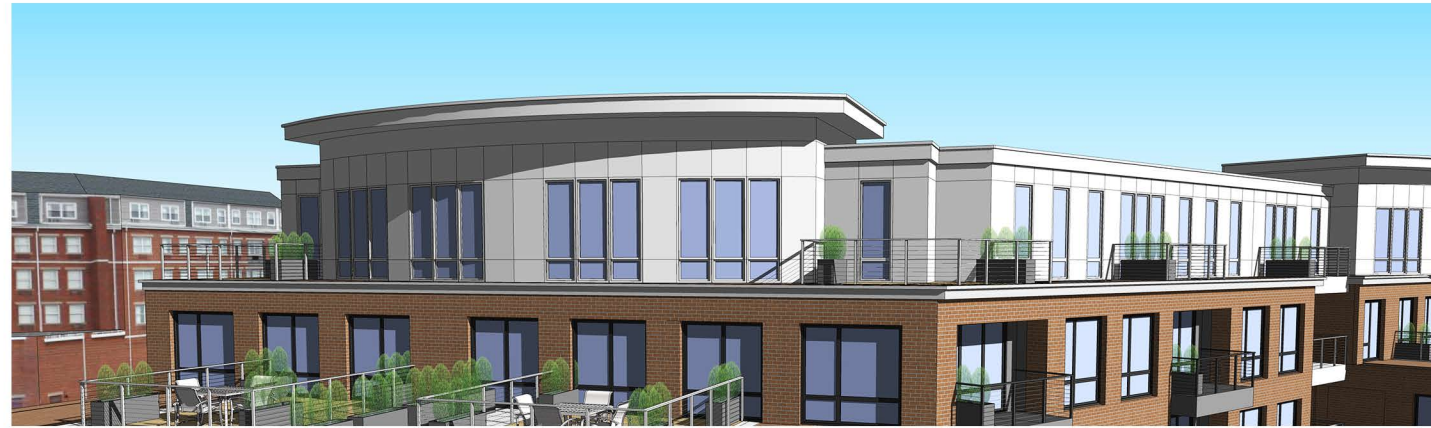
THIS CURVED NAUTICAL FOCAL POINT IS FLANKED WITH A RIBBON OF BALCONIES SET BACK FROM THE MASONRY FLOORS BELOW AND DEFINED BY A LIGHT HORIZONTAL RAIL DETAIL. ADDITIONAL ACCENT CAP BANDING HAS BEEN ADDED TO THE INSET RIBBON. THE OVERHANG AND CAP ON THE RADIAL FORMS HAVE ADDITIONAL EDGE DETAIL AND PANELS FURTHER DEFINE THE BUILDING TEXTURE.
