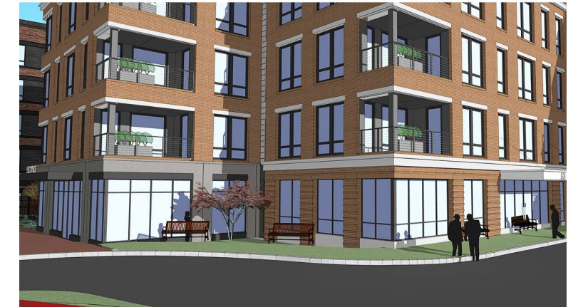
RESIDENTIAL AND COMMERCIAL BASE FORMS ARE DEFINED BY TWO DISTINCTLY DIFFERENT DESIGN STYLES. HORIZONTAL BRICK DETAILING HAS BEEN ADDED TO REFLECT THE HORIZONTAL SIDING ABOVE
