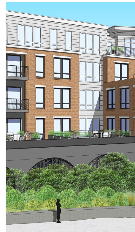
RECESSED BALCONY RIBBONS EXTEND THE VERTICAL SIDING ELEMENT DOWN TO REST ON A SOLID ARCHED BASE. DECORATIVE GRILLWORK PROVIDES A BACKDROP FOR THE LANDSCAPED EARTH BERM AND LOW SEATING WALL.
