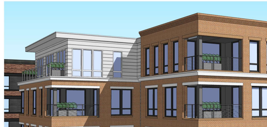
HORIZONTAL SIDING THEME CONTINUES AROUND THE FRONT, AND LINTEL DETAILS WRAP CORNER BALCONIES. BRICK CORBELING HAS BEEN ADDED TO THE TOP FLOOR TO COMPLEMENT THE TOP FLOOR SOLDIER COURSE AT THE WINDOW HEADS.
