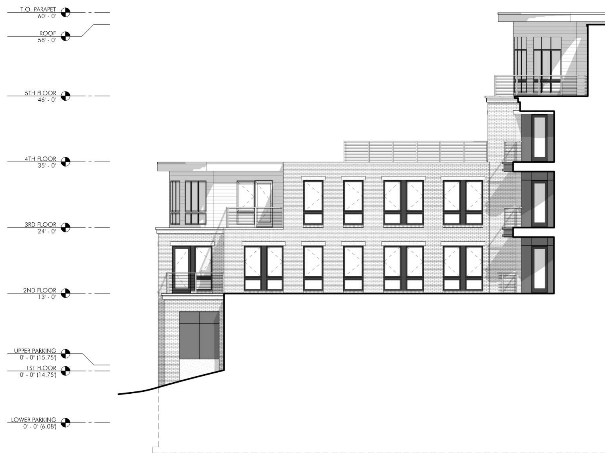
2 NORTH ELEVATION - WING 1/8" = 1'-0"
