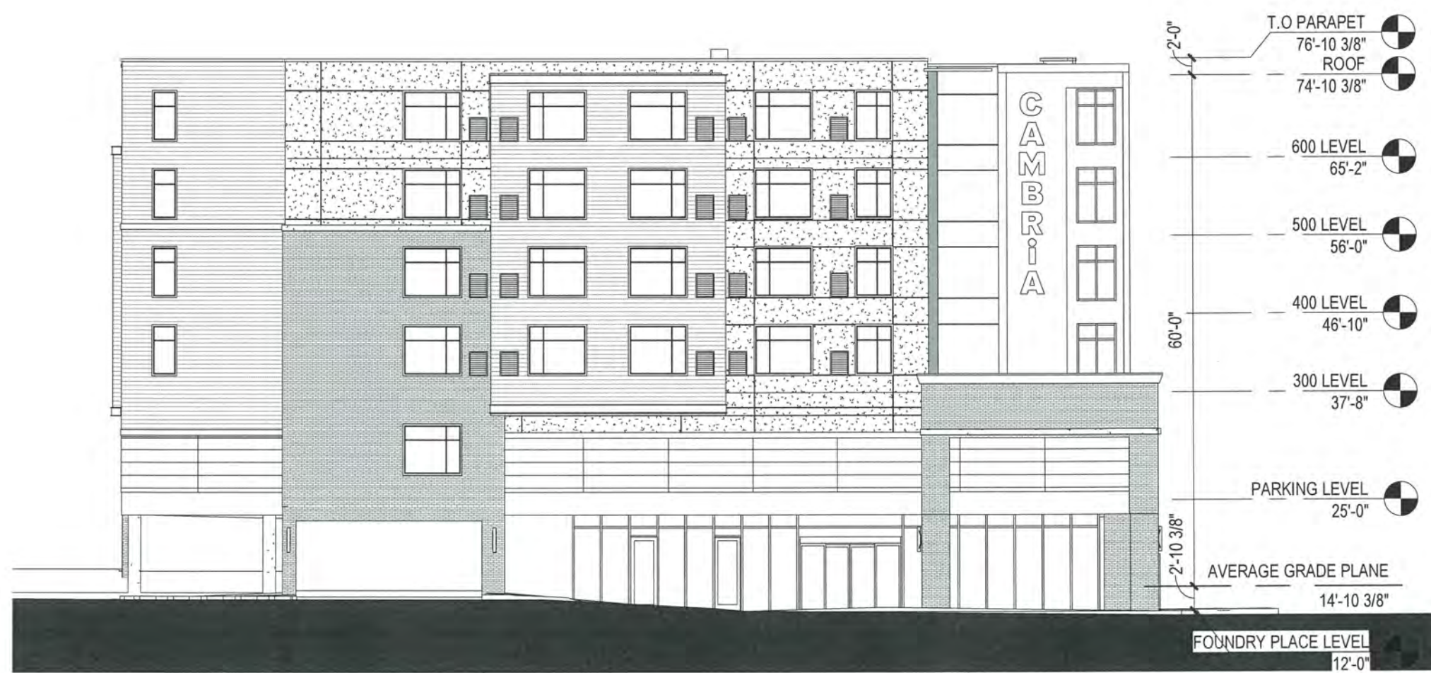
1 BUILDING ELEVATION - EAST 1/16" = 1'-0"
