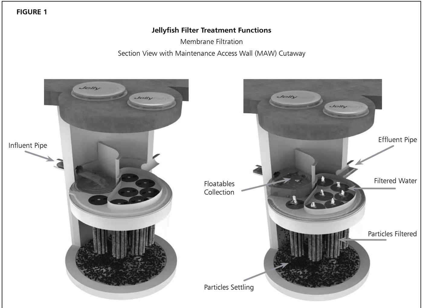
Jellyfish Filter cartridges are backwashed after each peak storm event, which removes accumulated sediment from the membranes. This backwash process extends the service life of the cartridges and increases the time between maintenance events.
