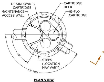
JELLYFISH TREATMENT CAPACITY IS A FUNCTION OF THE CARTRIDGE SELECTION AND THE NUMBER OF CARTRIDGES. THE STANDARD MANHOLE STYLE IS SHOWN. Ø48" MANHOLE JELLYFISH PEAK TREATMENT CAPACITY IS 0.45 CFS. IF THE SITE CONDITIONS EXCEED 0.45 CFS AN UPSTREAM BYPASS STRUCTURE IS REQUIRED.
