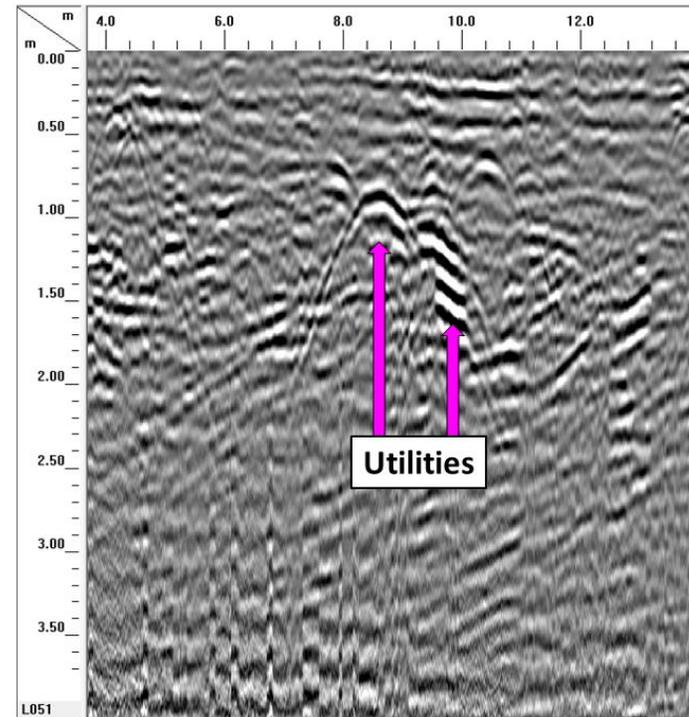
Figure 50: Selected GPR profile of the utilities located in Grid 3. The position of radar profile is indicated by the white arrow in the left plan view map, and the utilities are indicated by the magenta arrows in the radargram to the right.
