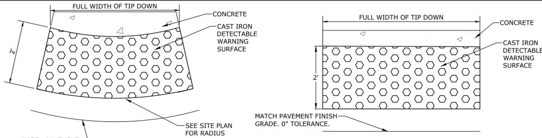
**CAST IRON DETECTABLE WARNING SURFACE**
