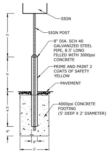
**BOLLARD MOUNTED SIGN DETAIL**
