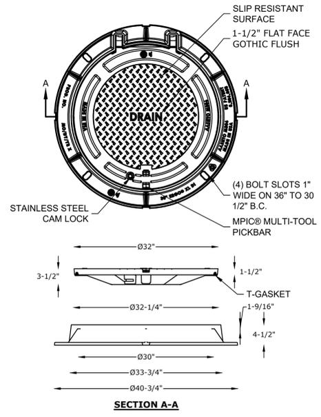
**DRAIN MANHOLE FRAME & COVER**
