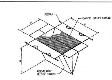
SILTATION BAG NOT TO SCALE USE "SILTSACK" AS MANUFACTURED BY ATLANTIC CONSTRUCTION FABRICS, INC. OR EQUIVALENT
