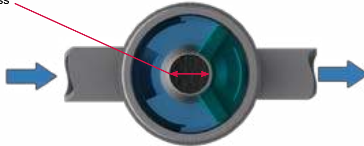
Fig.3 The central opening to the sump of the First Defense®-HC is 15 inches in diameter.
