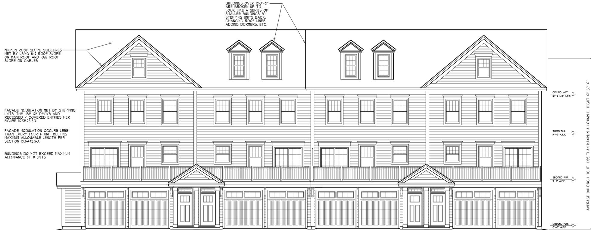
GATEWAY TOWNHOUSE: SHALL FOOTPRINT ATTACHED SINGLE FAMILY RESIDENTIAL BUILDINGS HAVE A NARROW MASSING AND MAY BE LOCATED ON INDIVIDUAL OR COMMON LOTS. EACH UNIT IS SEPARATED HORIZONTALLY BY A COMMON WALL.
