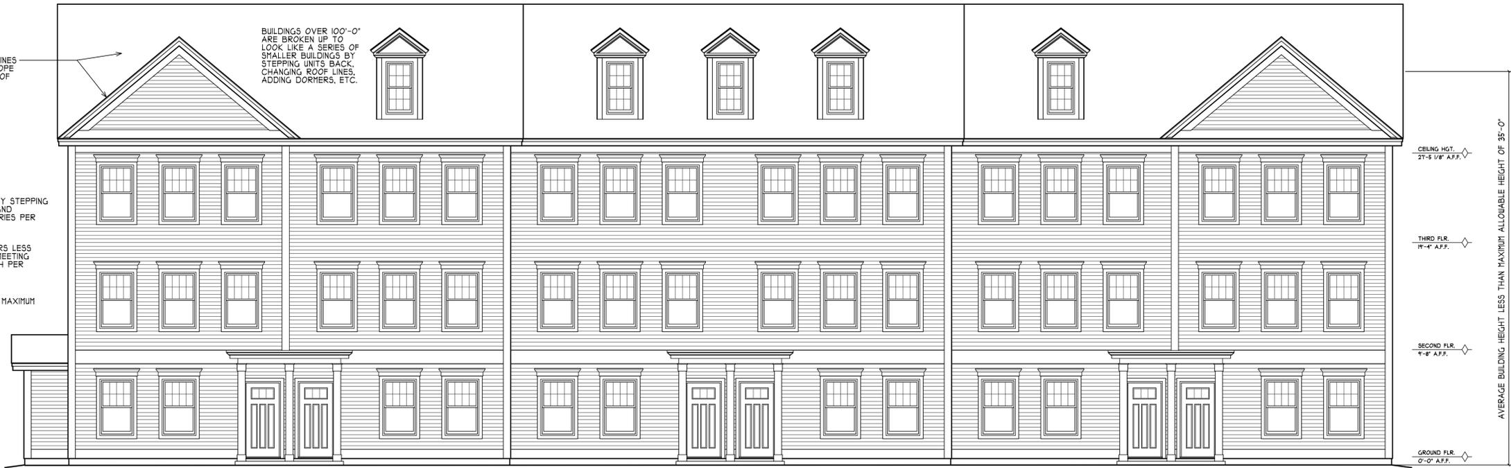
GATEWAY TOWNHOUSE: SMALL FOOTPRINT ATTACHED SINGLE FAMILY RESIDENTIAL BUILDINGS HAVE A NARROW MASSING AND MAY BE LOCATED ON INDIVIDUAL OR COMMON LOTS. EACH UNIT IS SEPARATED HORIZONTALLY BY A COMMON WALL.
