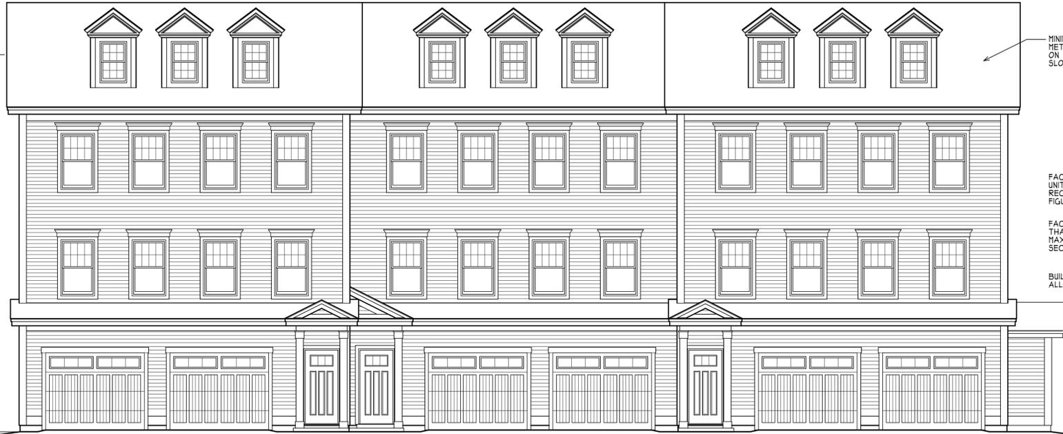
MINIMUM ROOF SLOPE GUIDELINES MET BY USING 8:12 ROOF SLOPE ON MAIN ROOF AND 10:12 ROOF SLOPE ON GABLES
