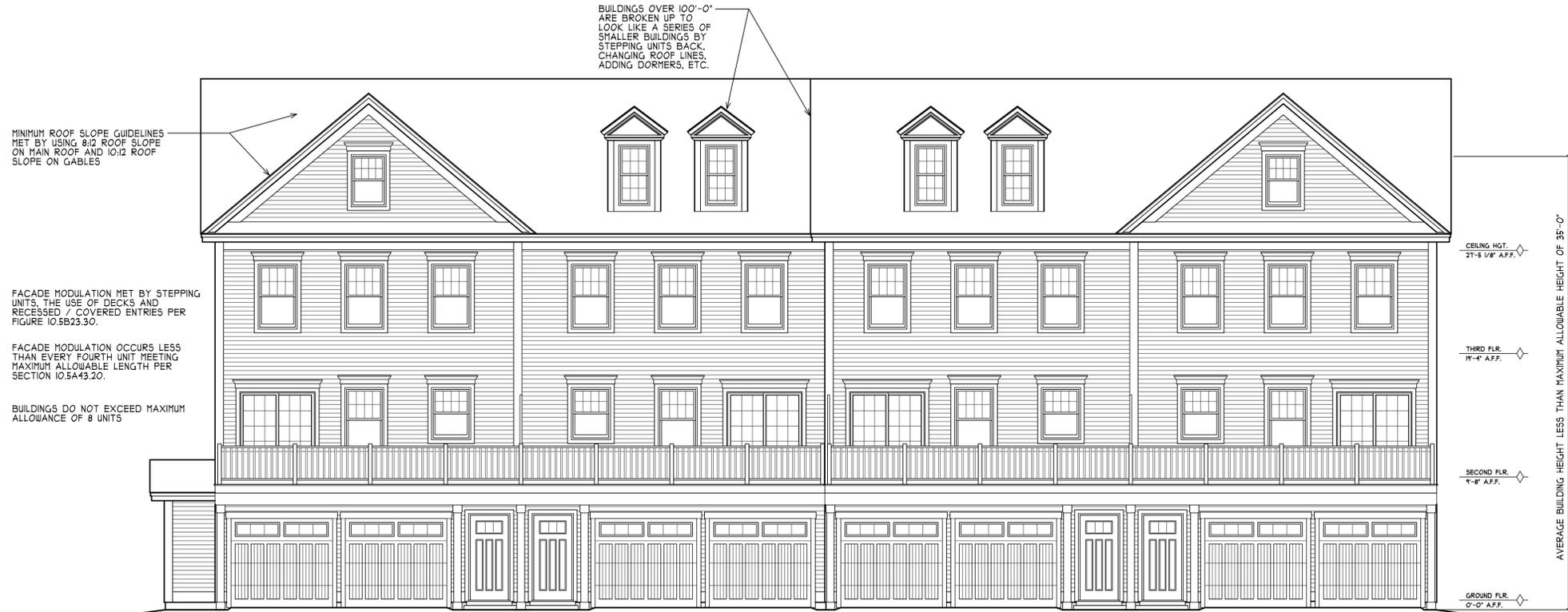
MINIMUM ROOF SLOPE GUIDELINES MET BY USING 8:12 ROOF SLOPE ON MAIN ROOF AND 10:12 ROOF SLOPE ON GABLES
