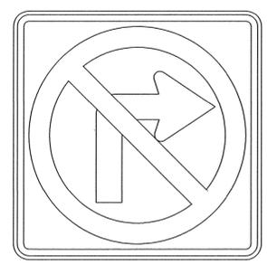
SIGN TO BE MOUNTED SO BOTTOM EDGE IS NO LESS THAN 7 FEET FROM GROUND SURFACE AND EDGE NEAREST STREET IS NO LESS THAN 2 FEET LATERALLY FROM EDGE OF PAVEMENT.
