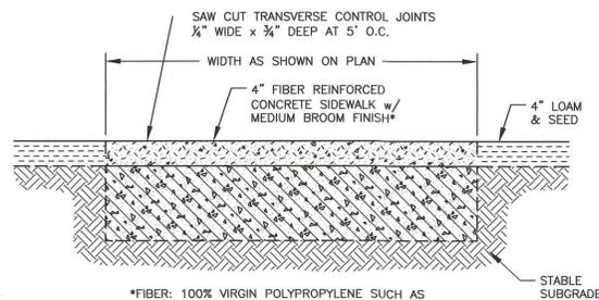
\*FIBER: 100% VIRGIN POLYPROPYLENE SUCH AS GRACE MICROFIBER, ASTM C116, TYPE 111, PAR.4.1.3. OR EQUAL APPLIED AT 1 LB. PER C.Y.
