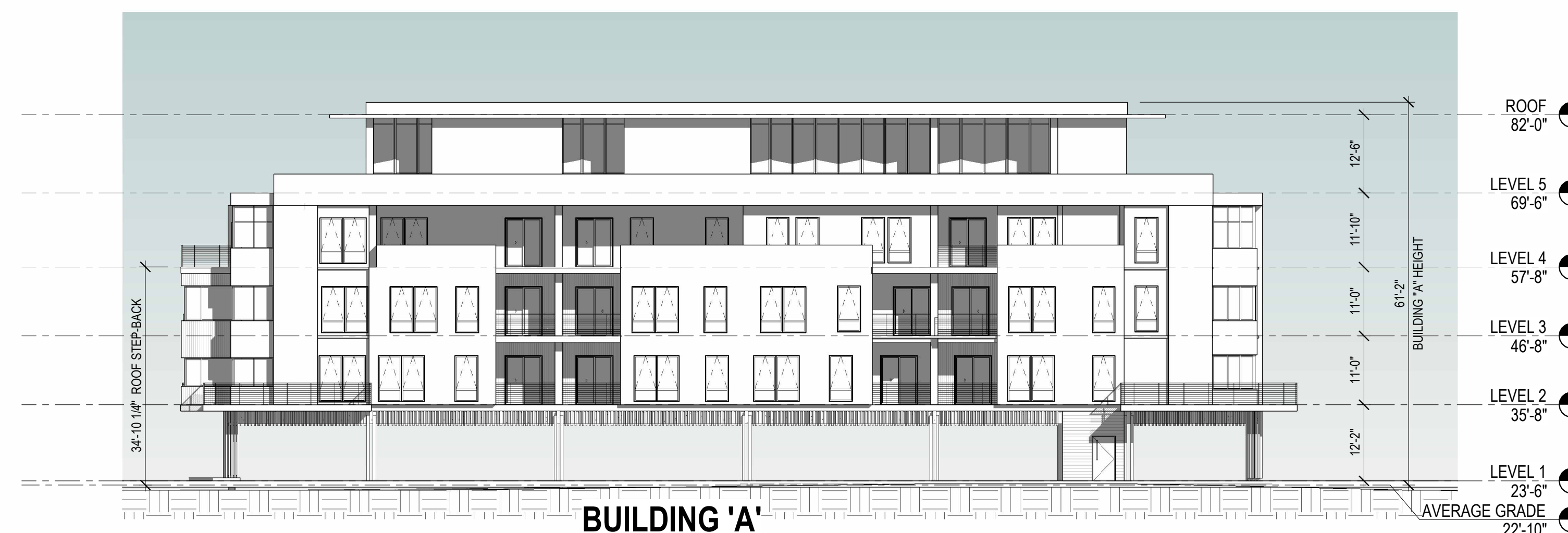
1 SOUTH ELEVATION PB 1/16" = 1'-0"
