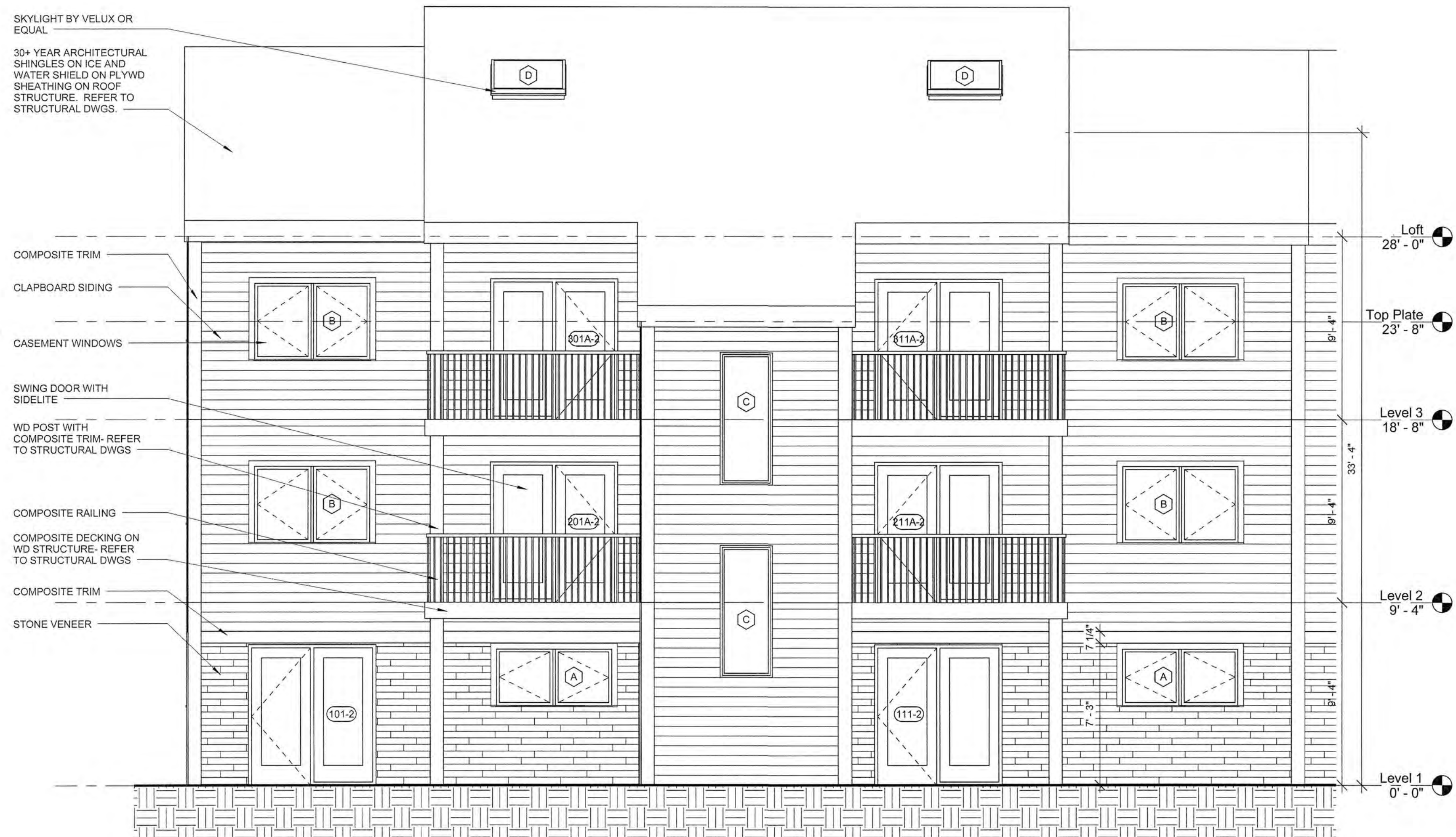
2 BUILDING 2- FRONT ELEVATION - ENLARGED VIEW 1/4" = 1'-0"
