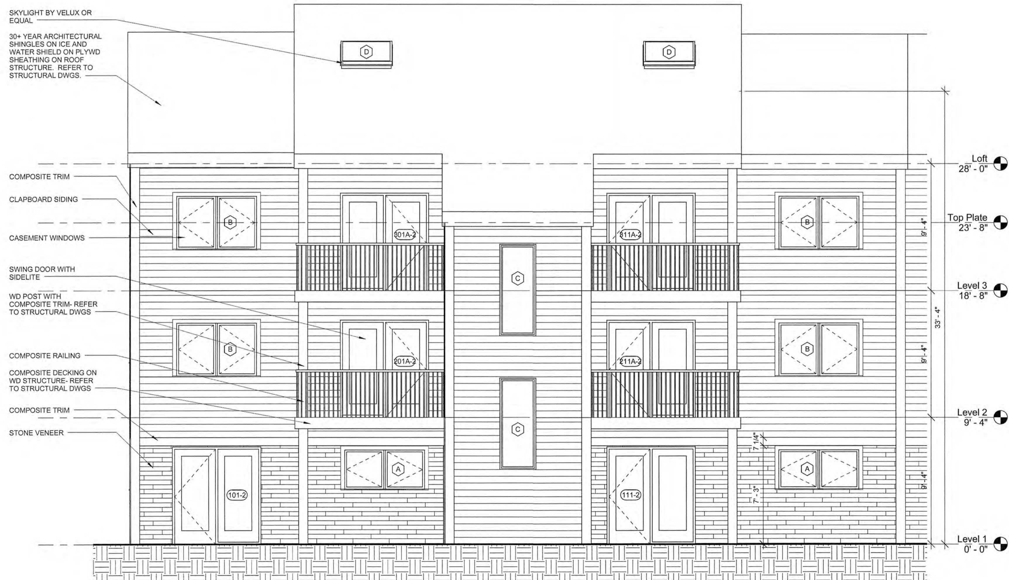
2 BUILDING 2- FRONT ELEVATION - ENLARGED VIEW 1/4" = 1'-0"
