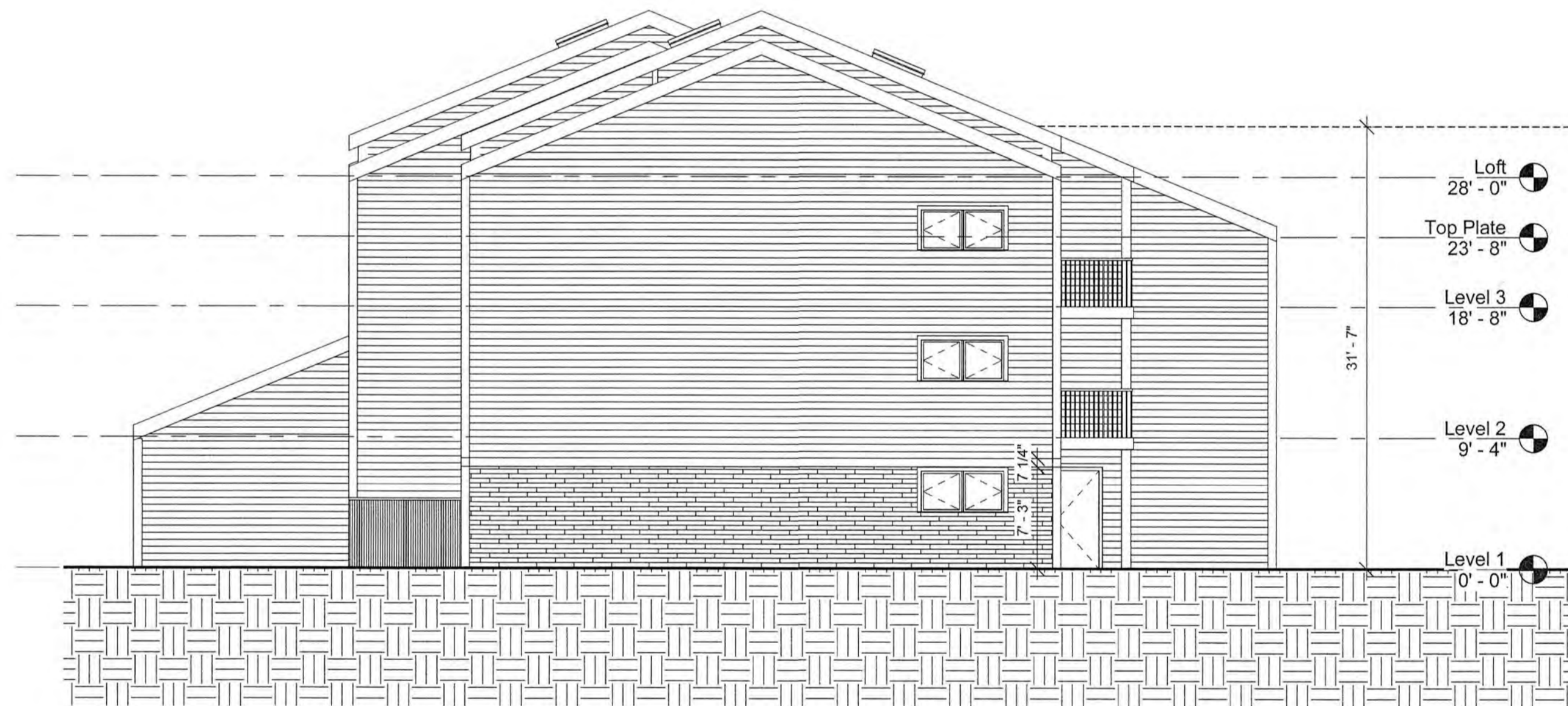
3 BUILDING 2 - WEST ELEVATION 1/8" = 1'-0"
