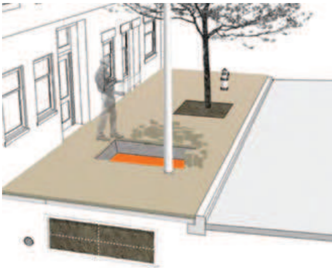
Utility access with pavers, step 1
