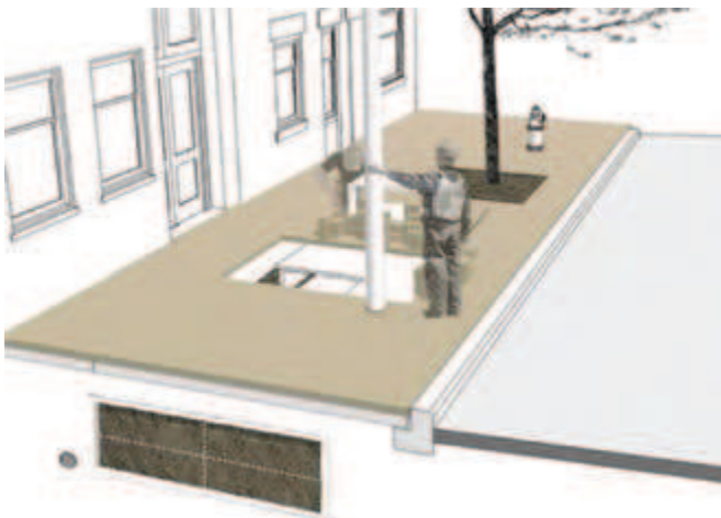
Utility access with pavers, step 2
