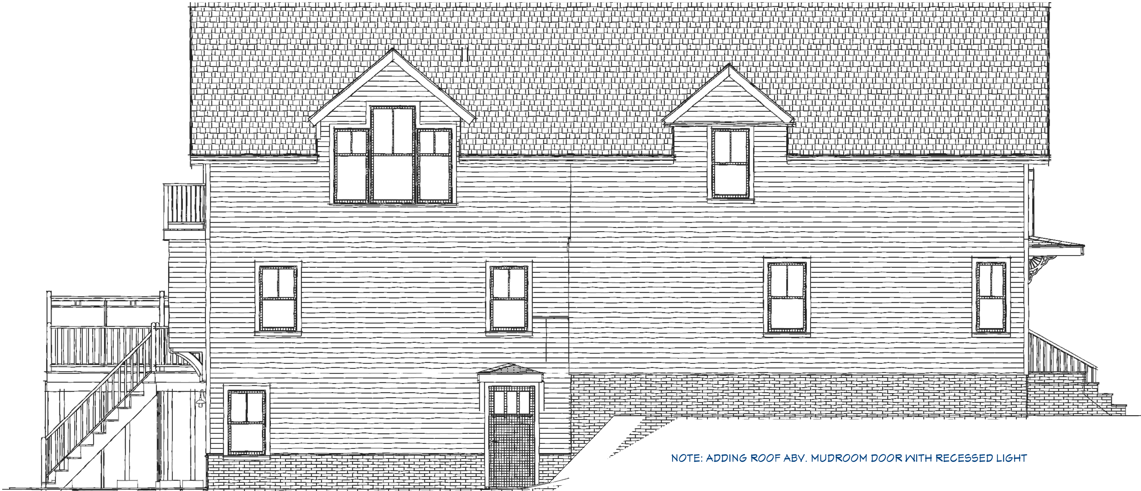
WEST PROPOSED ELEVATION | SIDEVIEW SCALE: 1/4" = 1'-0"
