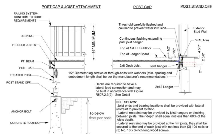
**Deck Ledger Attachment Detail for Step Down**
