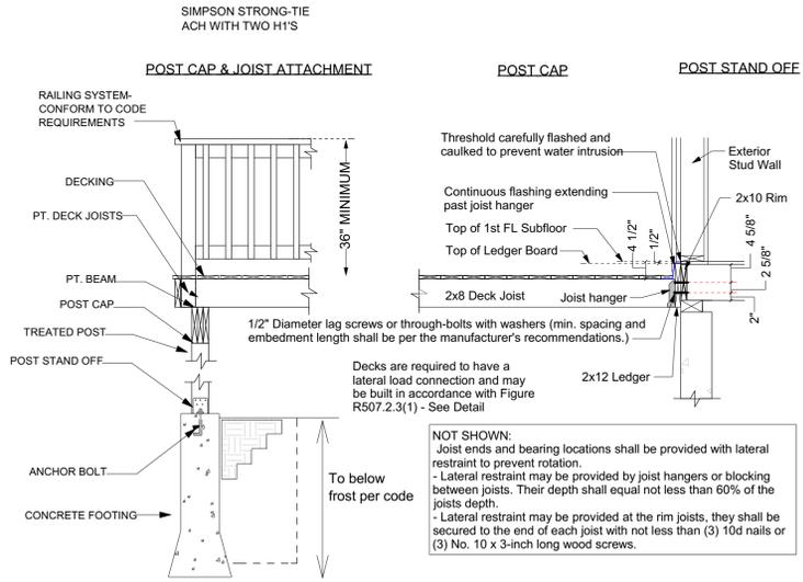
Deck Ledger Attachment Detail for Step Down
