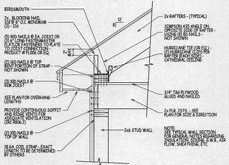
**ROOF THRUST CONNECTION DETAIL**
