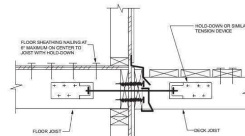
NOTE: hold down tension devices shall be installed in not less than 2 locations per deck, within 24 inches of each end of the deck. Each device shall have an allowable stress design capacity of not less than 1,500 lbs.
