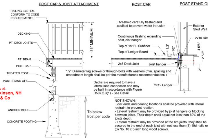
Deck Ledger Attachment Detail for Step Down
