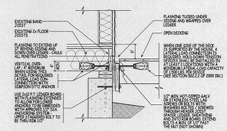
**DECK DETAIL - STEP DN. OPTION CONNECTION**
