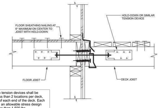
**FIGURE R507.2.3(2) DECK ATTACHMENT FOR LATERAL LOADS**
