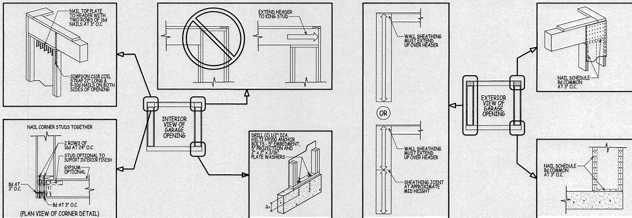
**APA NARROW WALL BRACING METHOD FRAMING TIPS (FORM F435)**
