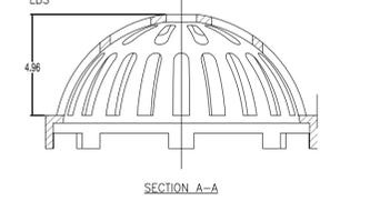
DIMENSIONS ARE FOR REFERENCE ONLY ACTUAL DIMENSIONS MAY VARY DIMENSIONS ARE IN INCHES QUALITY: MATERIALS SHALL CONFORM TO ASTM A536 GRADE 70-50-05 PAINT: CASTINGS ARE FURNISHED WITH A BLACK PAINT LOCKING DEVICE AVAILABLE UPON REQUEST
