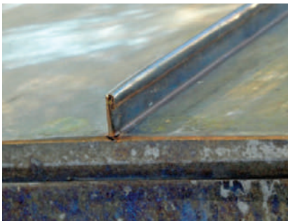
10 months exposure in a Northeastern coastal environment
