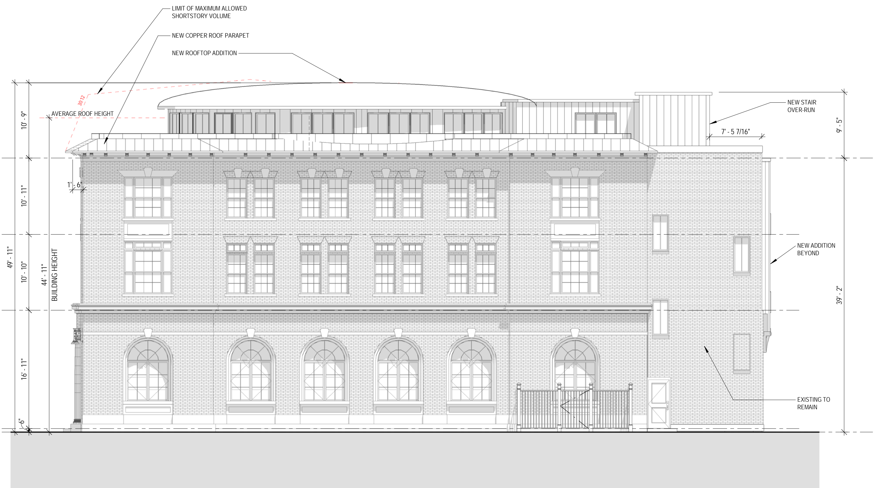
2 SIDE (SOUTH) ELEVATION - PROPOSED 1/8" = 1'-0"
