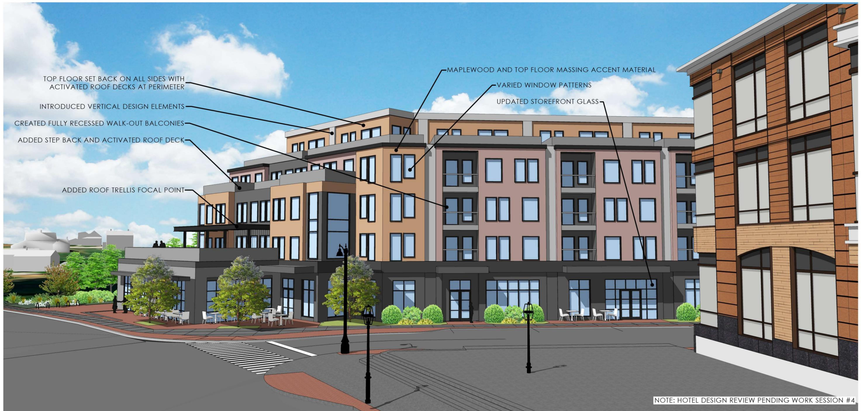
TOP FLOOR SET BACK ON ALL SIDES WITH ACTIVATED ROOF DECKS AT PERIMETER
