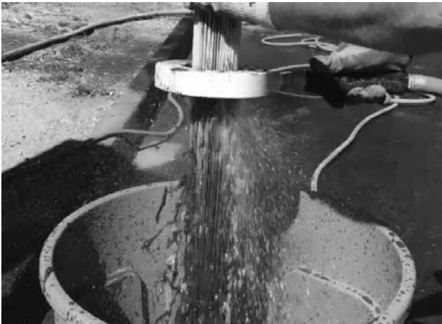
Rinsing Cartridge with Contech Rinse Tool
