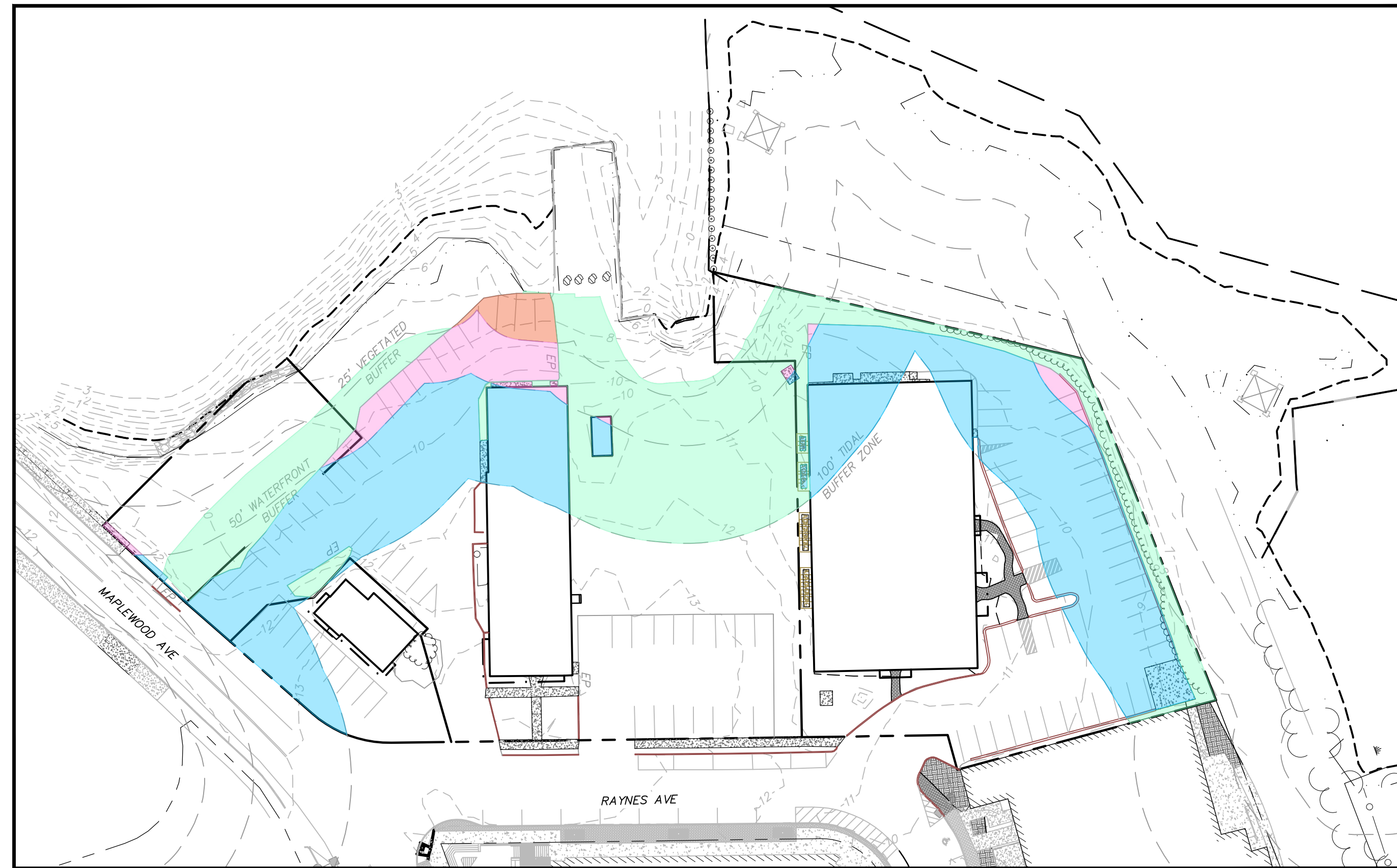
EXISTING CONDITIONS IMPERVIOUS SURFACE
