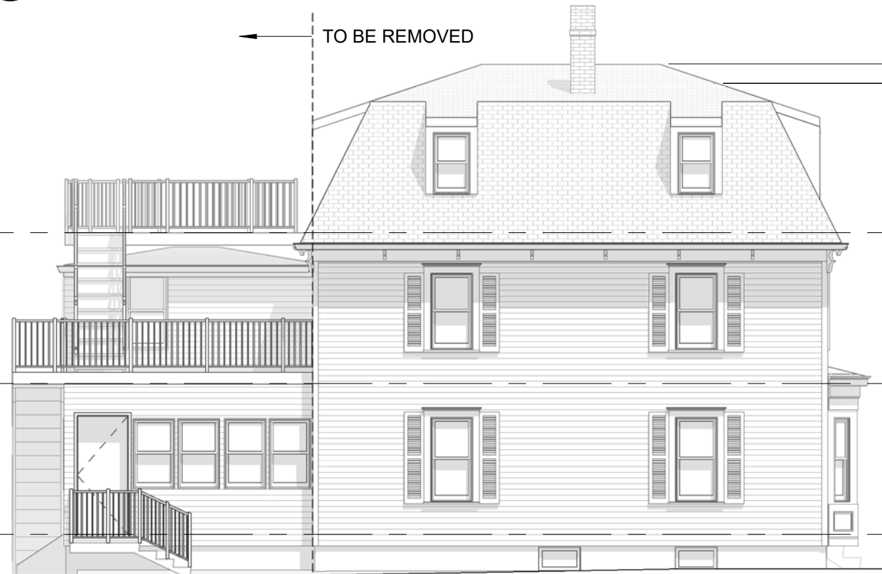
4 EXISTING SOUTH ELEVATION 1/8" = 1'-0"
