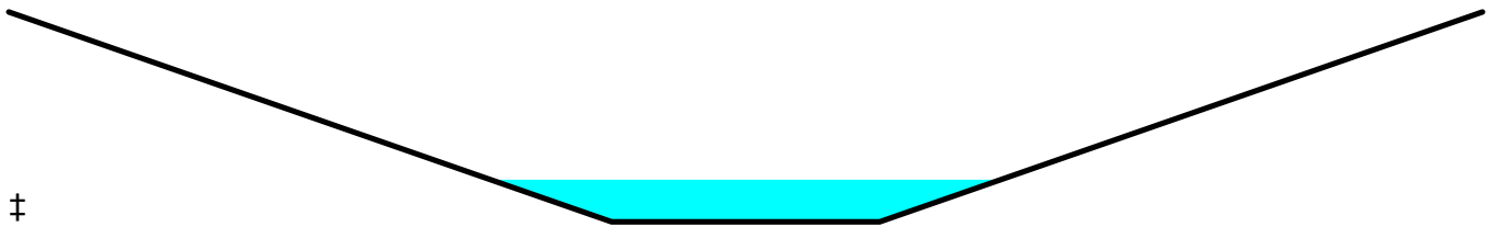
Reach R1: Swale
