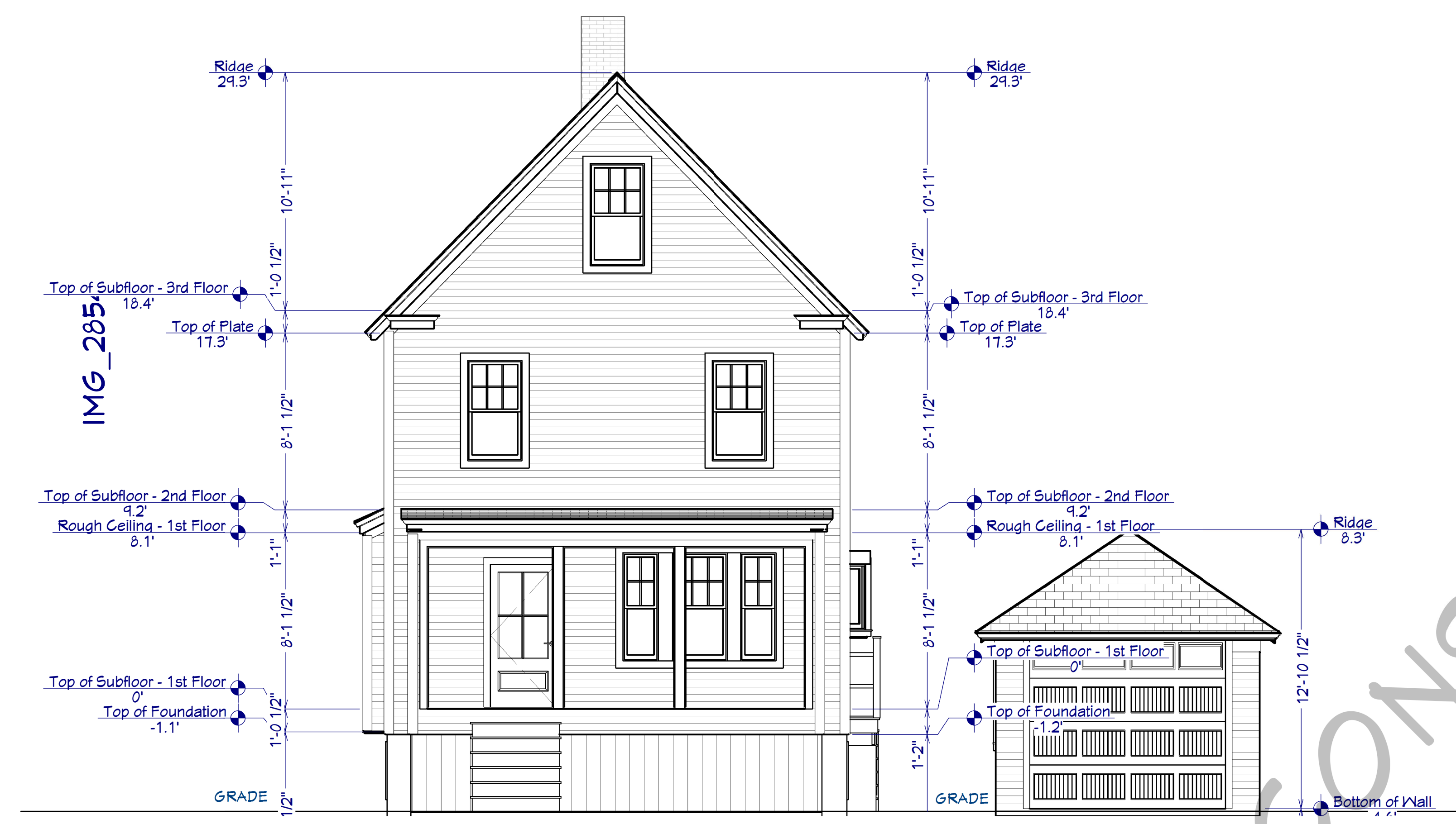
EXISTING NORTH ELEVATION | FRONT VIEW SCALE: 1/4" = 1'-0"
