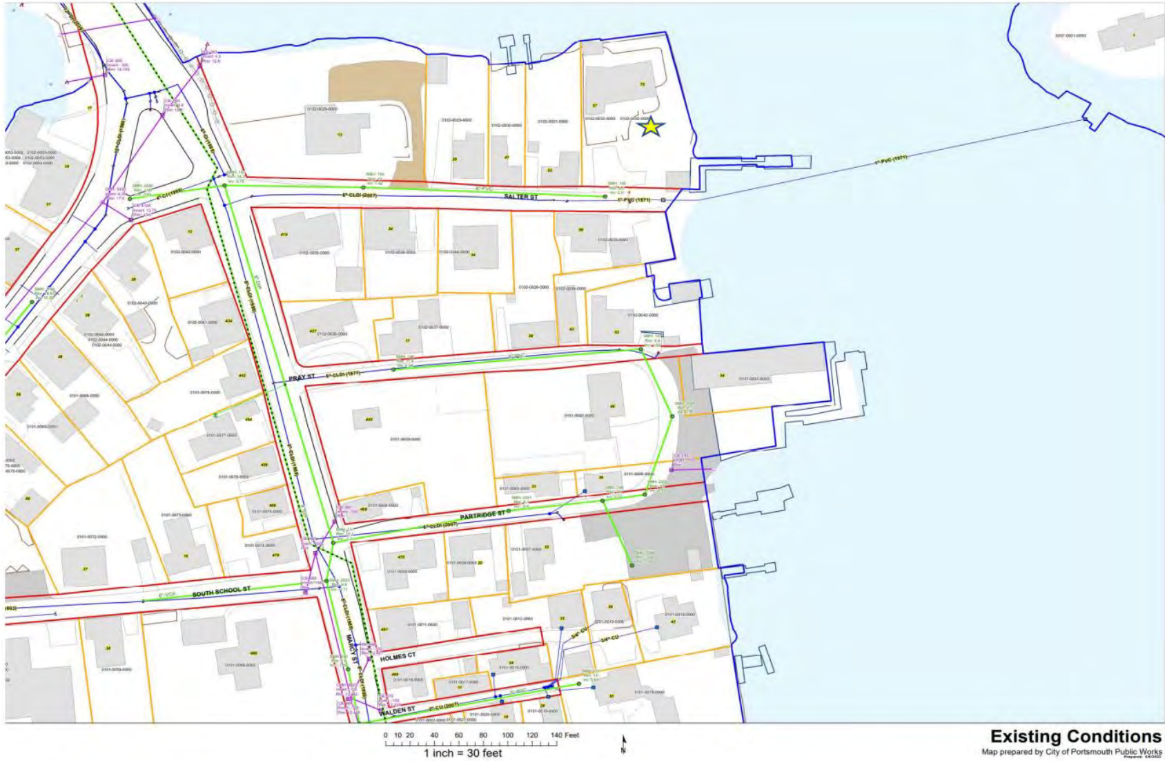
City of Portsmouth Public Works Map showing Water (Blue), Sewer (Green), and Drain (Purple) facilities in the area of 57 Salter Street (★)
