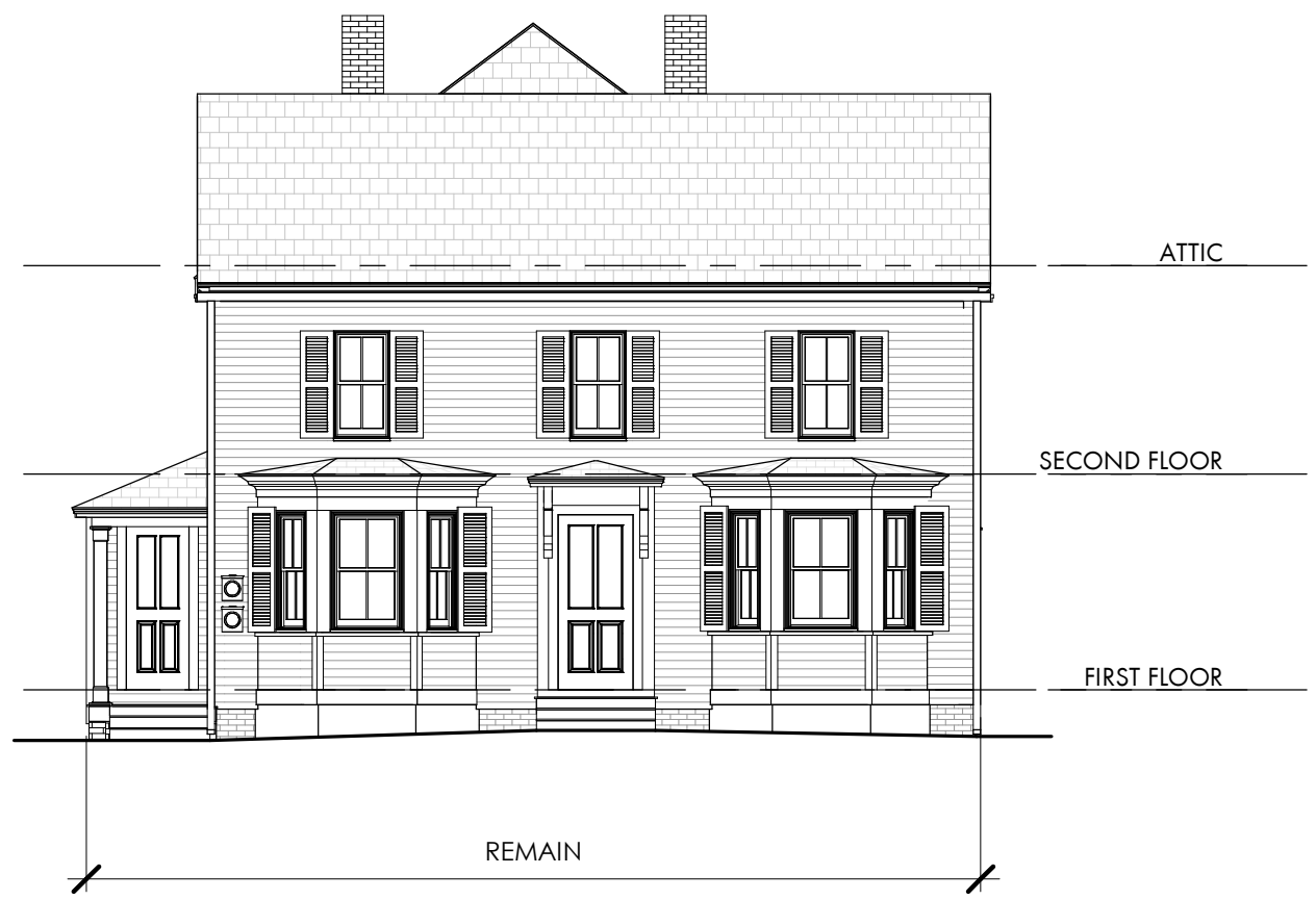
EXISTING WEST ELEVATION 2 1/8" = 1'-0"
