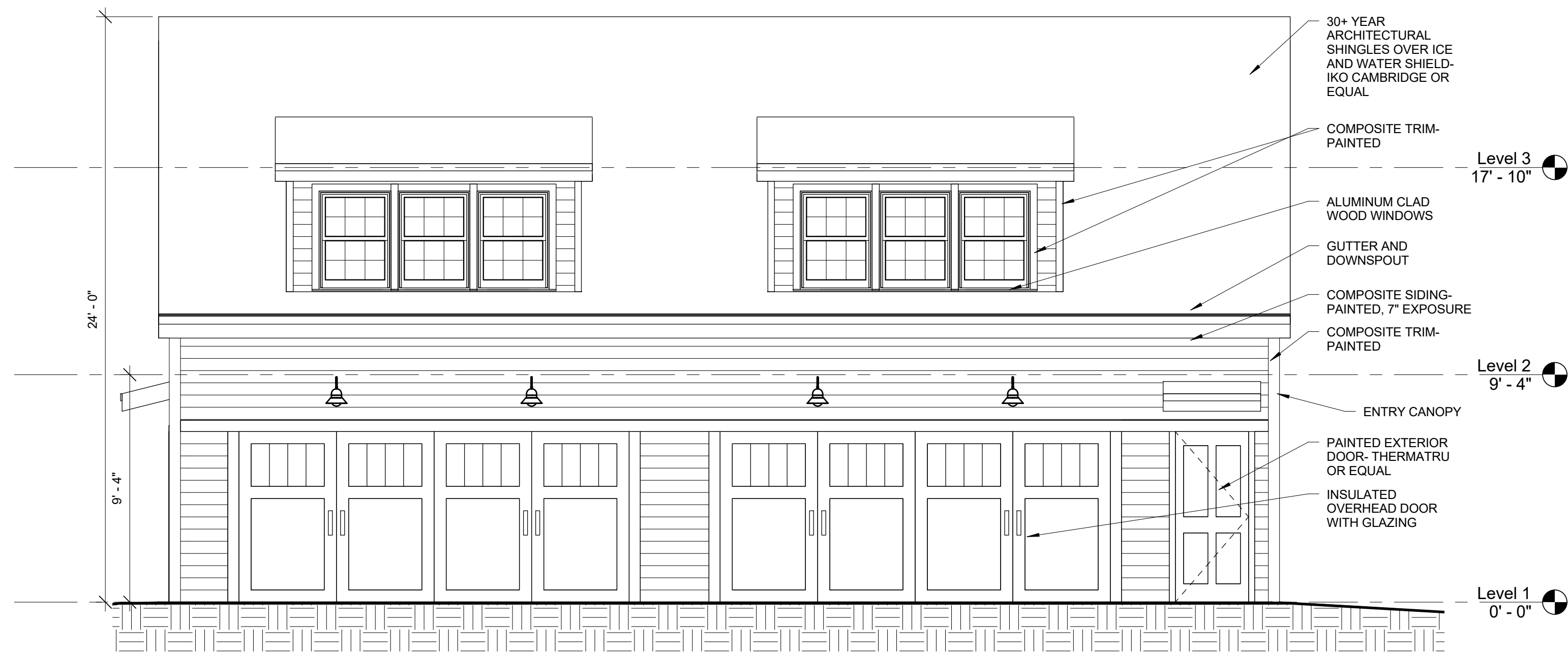
1 West Elevation- Apartment 1/4" = 1'-0"
