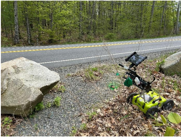
GPR Scanning North side of Wentworth Rd.
