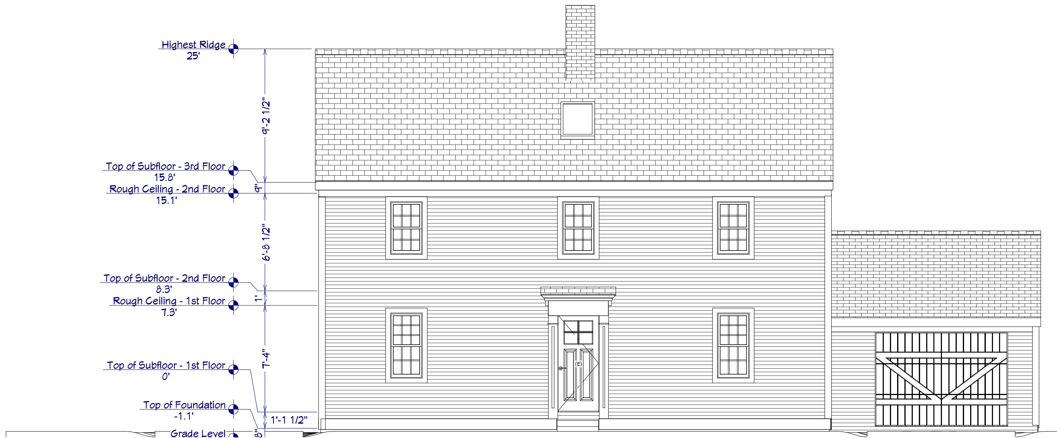
EXISTING TO REMAIN FRONT ELEVATION
