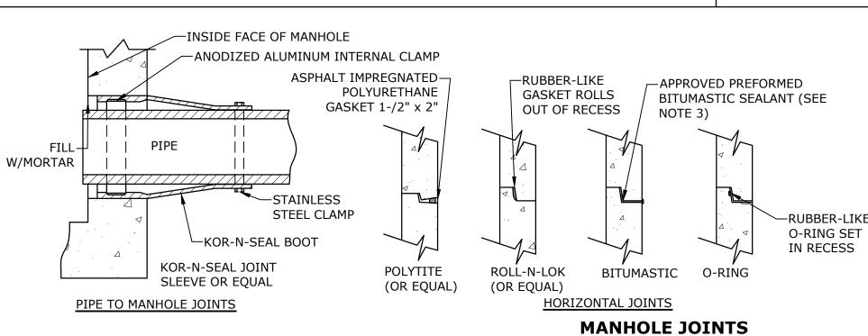
HORIZONTAL JOINTS BETWEEN THE SECTIONS OF PRECAST CONCRETE BARRELS SHALL BE PER CITY OF PORTSMOUTH DPW STANDARD AND SHALL BE SEALED FOR WATERTIGHTNESS USING A DOUBLE ROW ELASTOMERIC OR MASTIC-LIKE GASKET PIPE TO MANHOLE JOINTS SHALL BE PER CITY OF PORTSMOUTH STANDARD.
