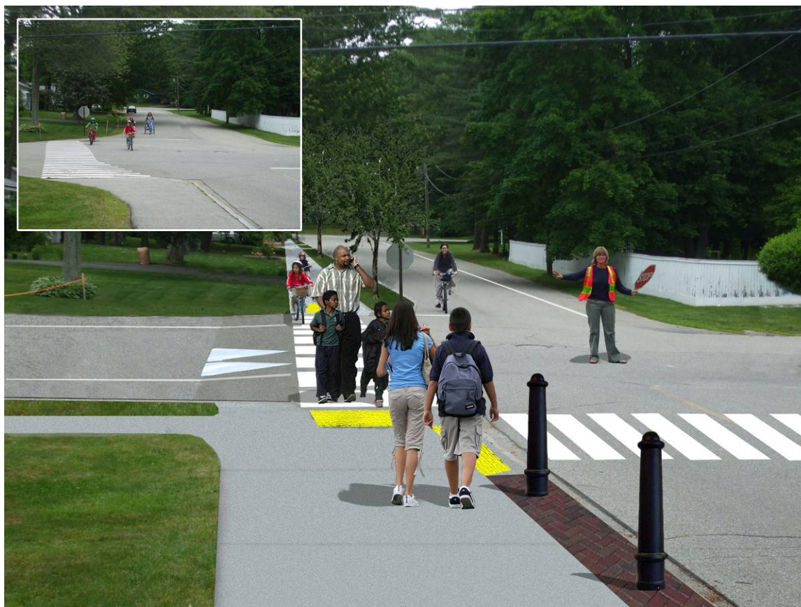
Fillmore Road and Van Buren Avenue Intersection improvements could include a raised crosswalk, new sidewalks and a wider sidewalk (foreground) leading to the school.
