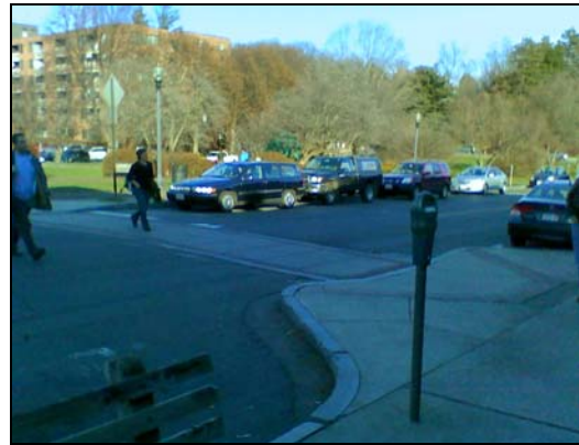
Bump outs help to slow traffic and reduce the crossing distance for pedestrians
