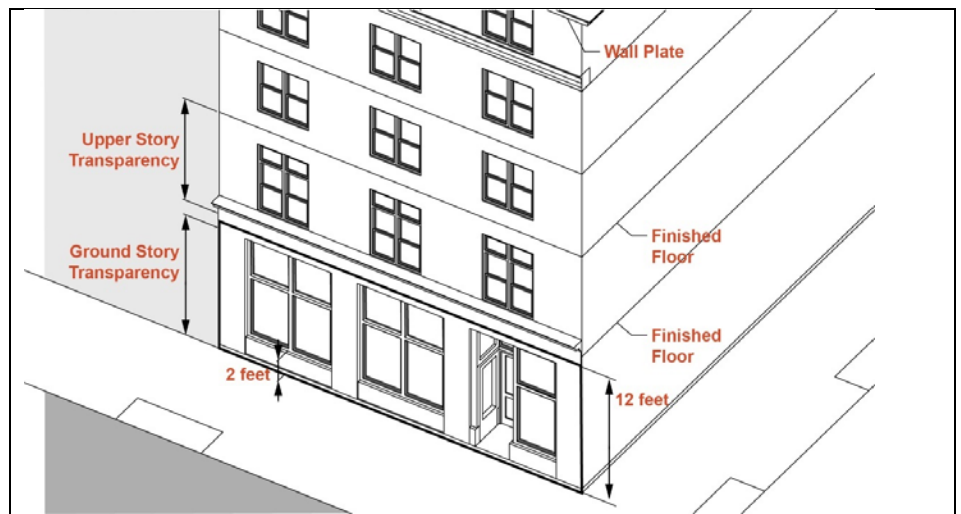
Figure 10.5B25.10 - Ground Floor and Upper Floor Façade Glazing
