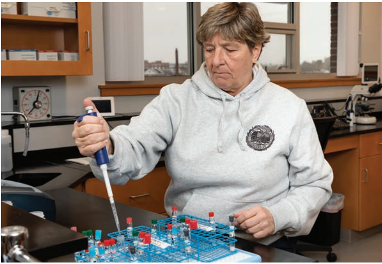
During the plant upgrade, an old biosolids processing building was converted to an operations center and a laboratory, where operator Kathy Sanborn is shown pipetting samples for nitrite, nitrate and ammonia using TNT vials (Hach).
