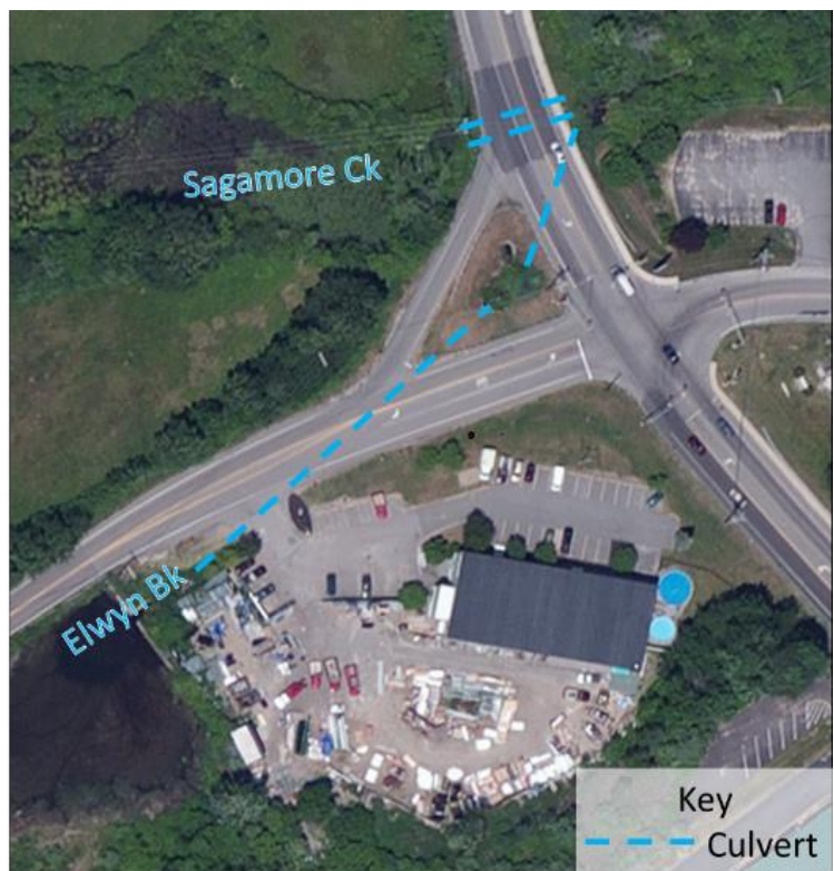
Depiction of flow routes for Sagamore Creek and Elwyn Brook through culverts under Banfield Road and Peverly Hill Road.
