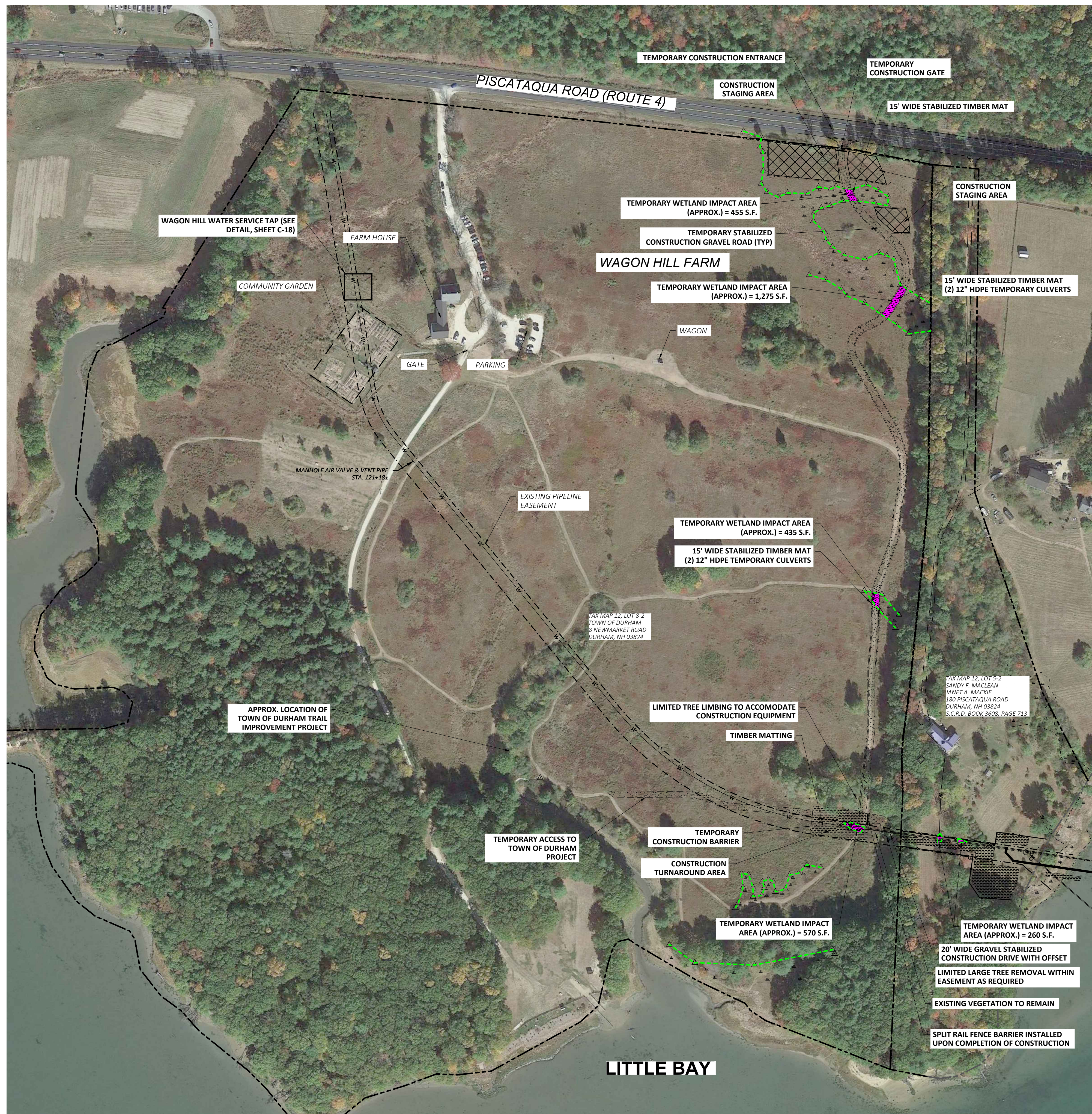
CONSTRUCTION ACCESS PLAN - DURHAM SCALE: 1"=125'
