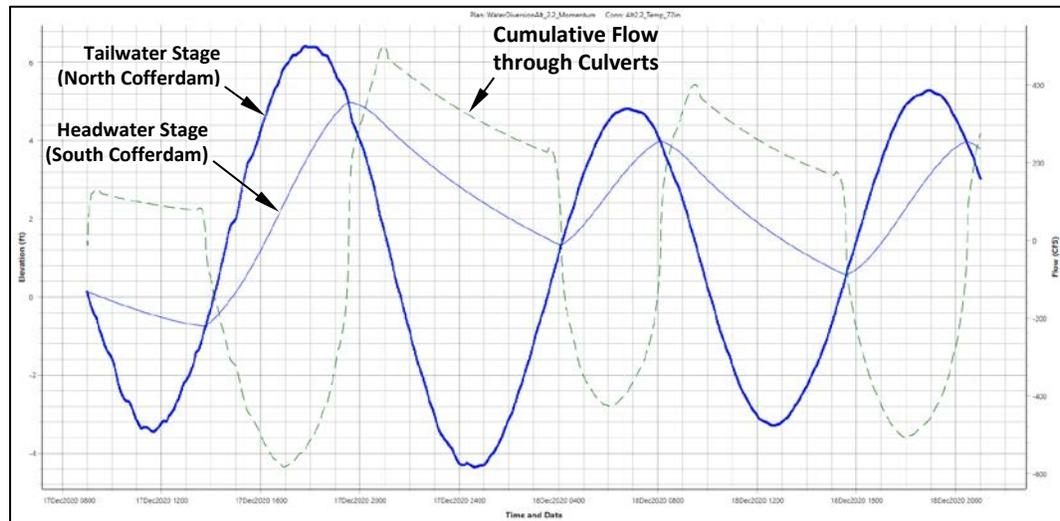
*Figure 42 – Stage and flow hydrographs calculated at the bridge for Water Diversion Alternative 2.2*
