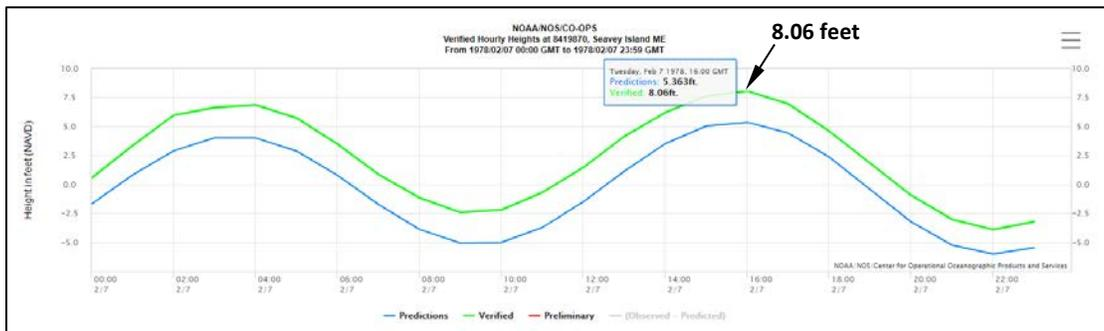
Figure 11 – Stage hydrograph showing water levels measured at the Seavey Island, ME tide gage on February 7, 1978. The green line represents measured water levels and the blue line represents predicted water levels.
