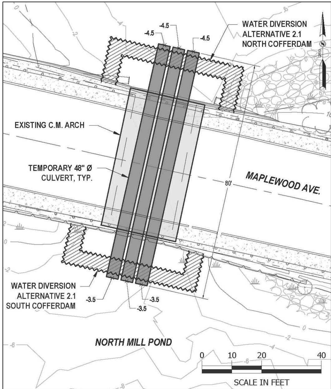
Figure 39 – Water Diversion Alternative 2.1 Schematic Plan
