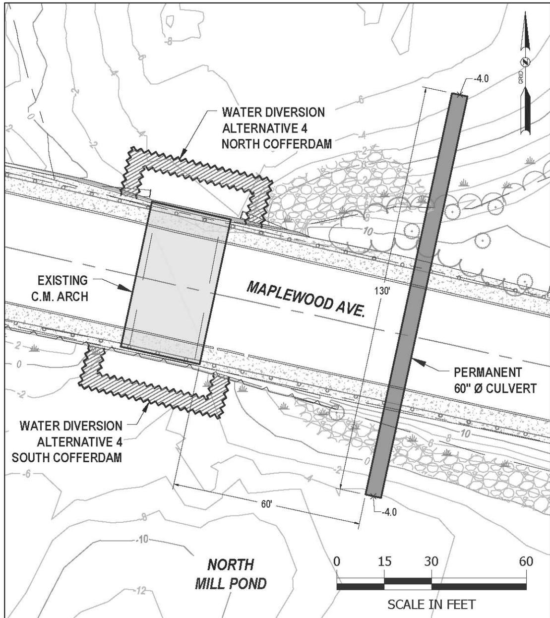
Figure 49 – Water Diversion Alternative 4 Schematic Plan
