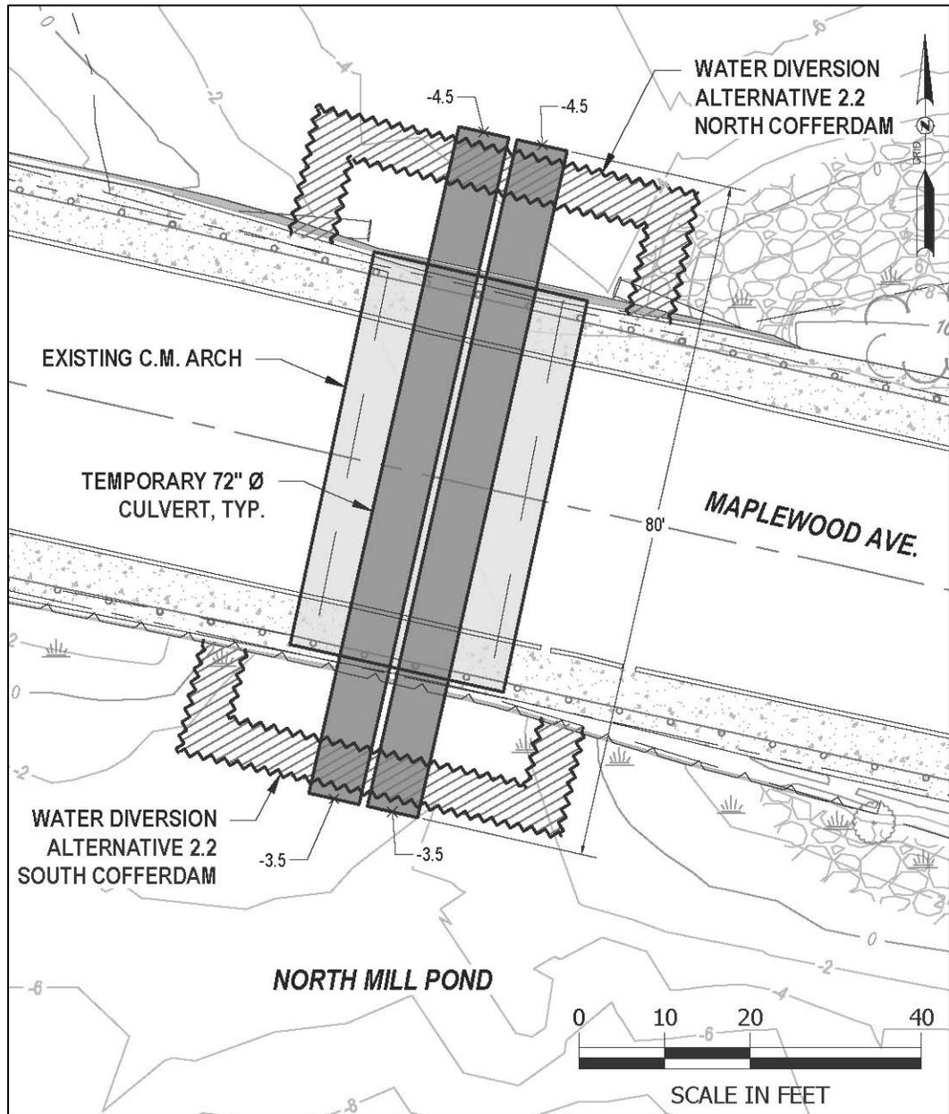
Figure 43 – Water Diversion Alternative 2.2 Schematic Plan
