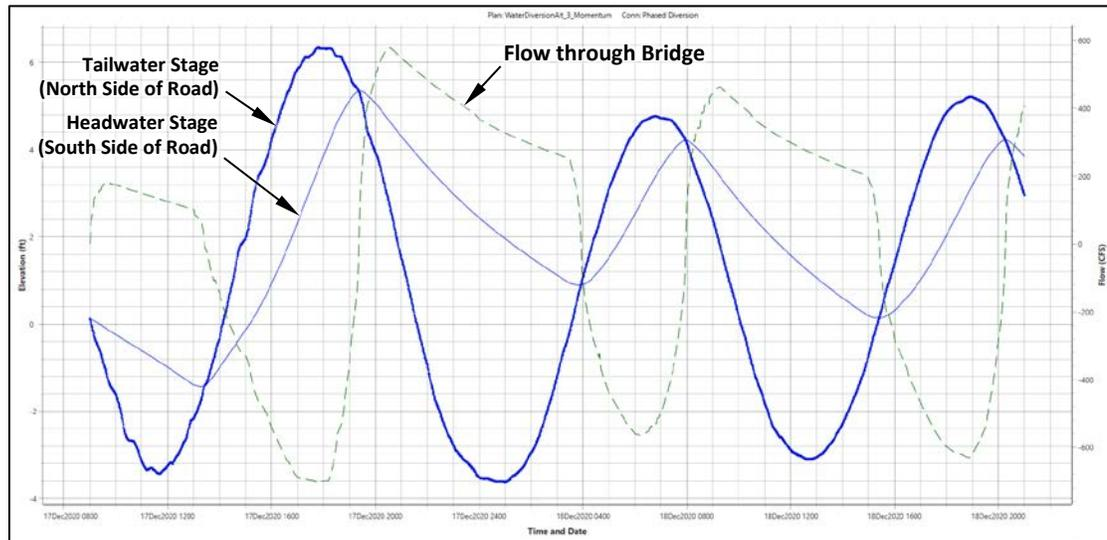
Figure 48 – Stage and flow hydrographs calculated at the bridge for Water Diversion Alternative 3
