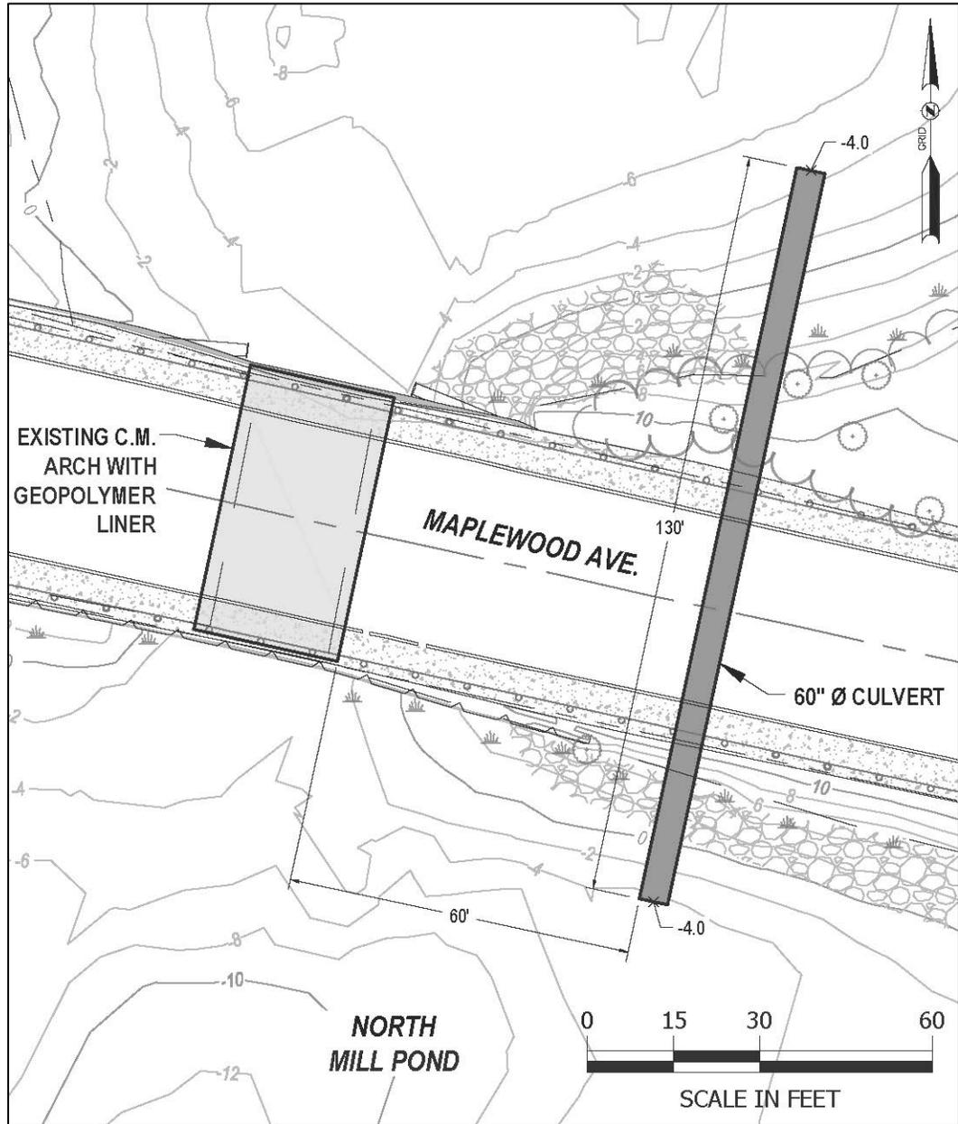
Figure 28 – Bridge Rehabilitation Alternative 2.2 schematic plan
