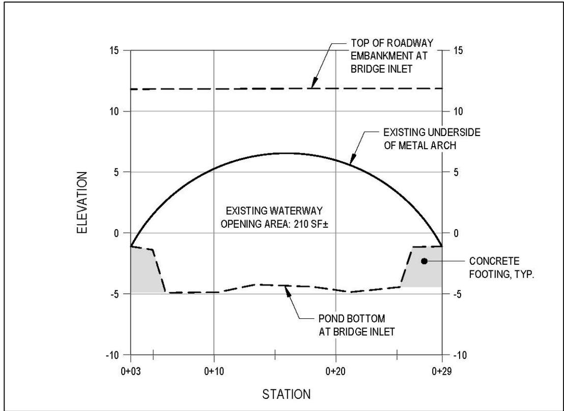
Figure 15 – Existing bridge inlet cross-section
