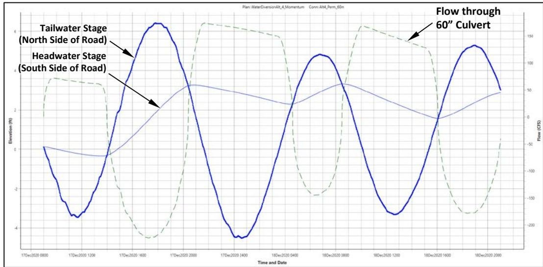
Figure 50 – Stage and flow hydrographs calculated for Water Diversion Alternative 4
