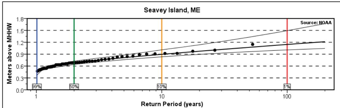
Figure 9 – High water annual exceedance probability curve for NOAA station 8419870 (Seavey Island, ME)
