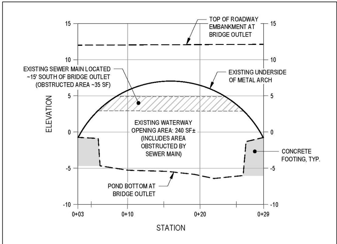
Figure 16 – Existing bridge outlet cross-section
