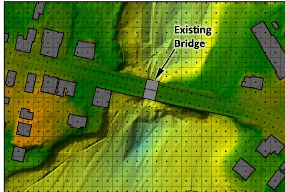
Figure 6 – Computational mesh in the vicinity of Maplewood Avenue used in the existing conditions hydraulic models
