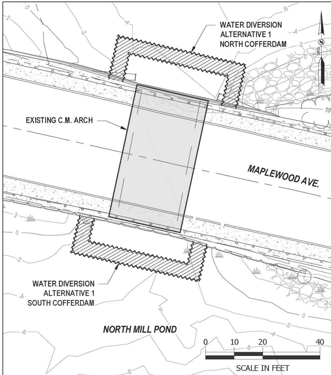
Figure 34 – Water Diversion Alternative 1 Schematic Plan
