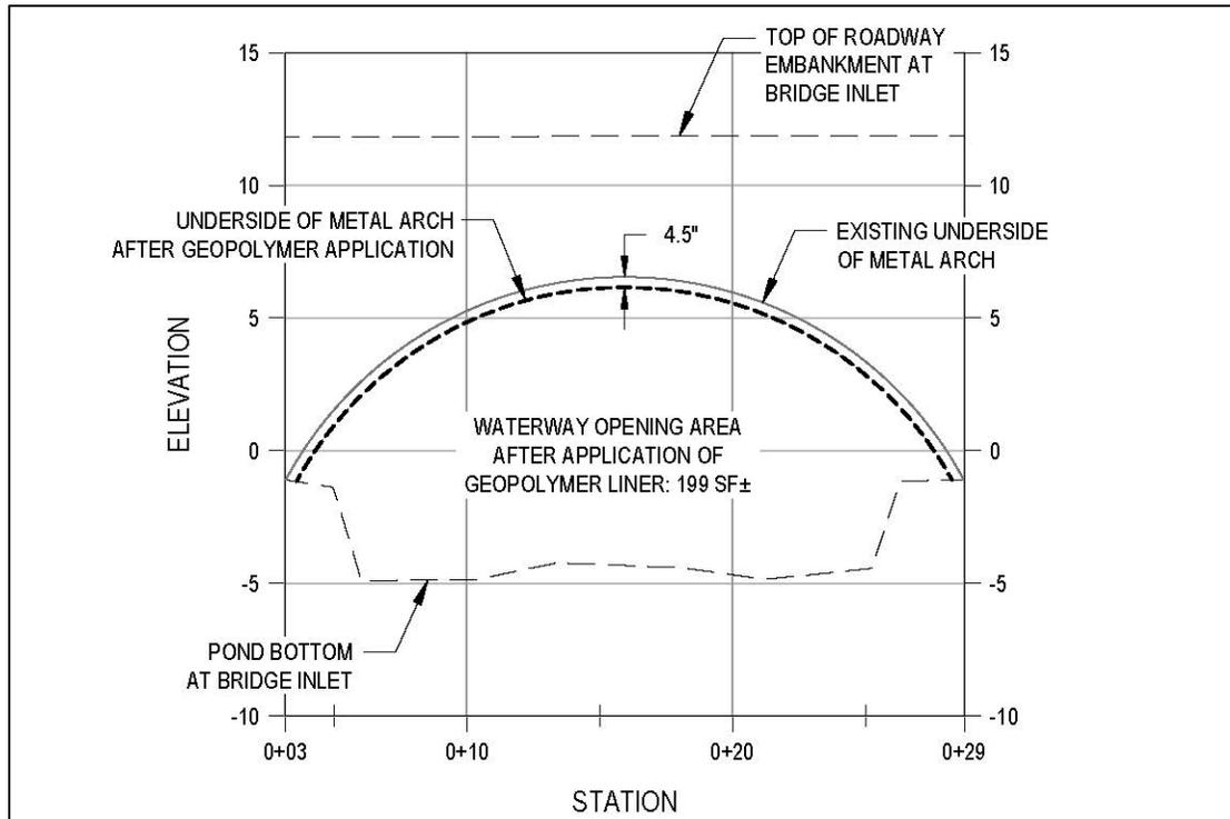
Figure 23 – Bridge Rehabilitation Alternative 1 inlet cross-section
