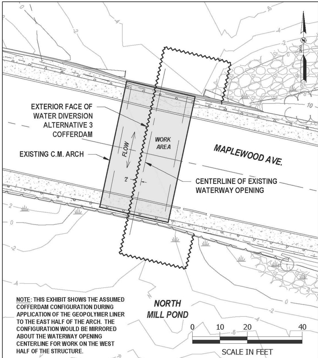
Figure 45 – Water Diversion Alternative 3 Schematic Plan
