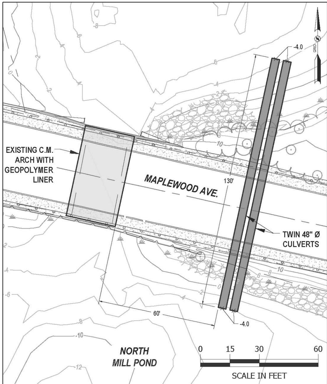
Figure 27 – Bridge Rehabilitation Alternative 2.1 schematic plan
