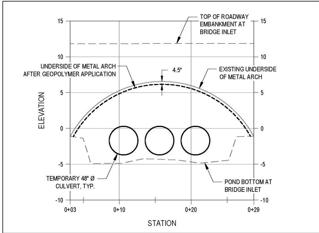
Figure 40 – Water Diversion Alternative 2.1 Bridge Inlet Cross-Section
